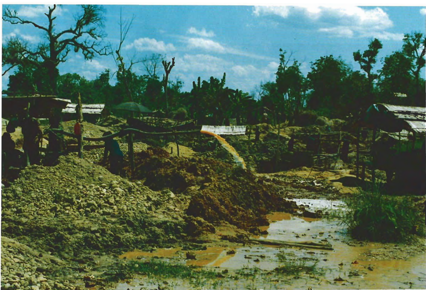
Figure 5. The Cempaka mining area is a jumble of shafts and tailings. When a pit is exhausted, the miners move a small distance to continue extracting the gem-bearing gravels. Because the upper gem gravels have been largely worked out, mining is more difficult and the miners are more likely to work as a team. Photo by David Dikinis.
