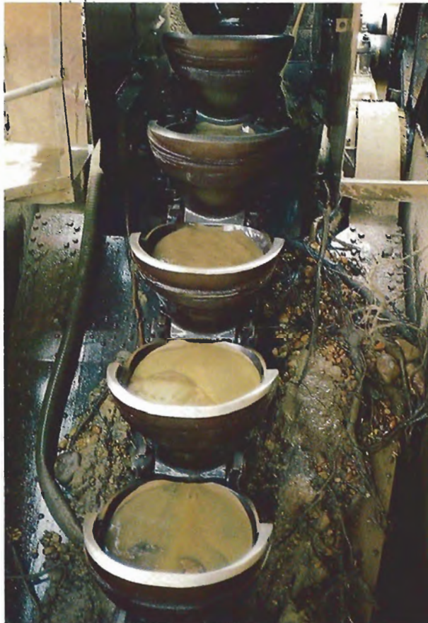
Figure 2. Dredge buckets on the Tejucana diamond dredge systematically scrape the river bottom and bring all of the material into the dredge for sorting. Photo by Kristi A. Koivula.
