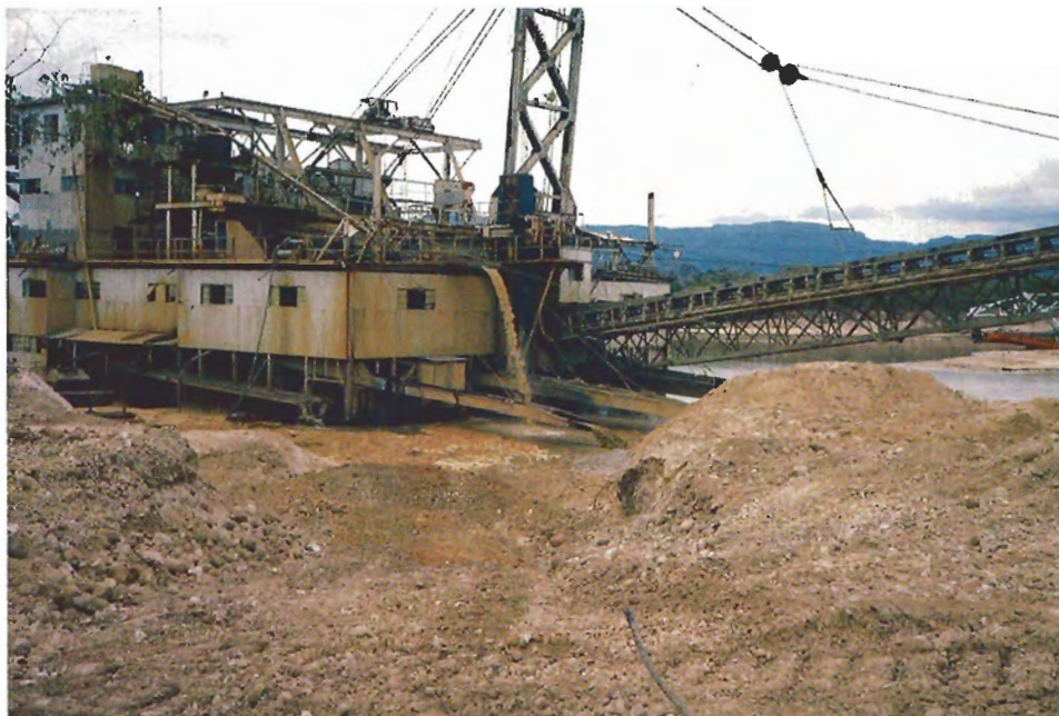
Figure 1. The Tejucana diamond dredge (here, operating near Diamantina, in Minas Gerais, Brazil) removes river gravels and mechanically sorts them for diamonds and gold. Photo by Kristi A. Koivula.
