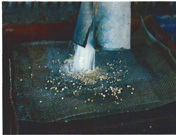
Figure 10. Material emitted from the jigs at the Acorn Securities sampling plant will be further examined by hand for diamond rough. Photo by David Dikinis.
