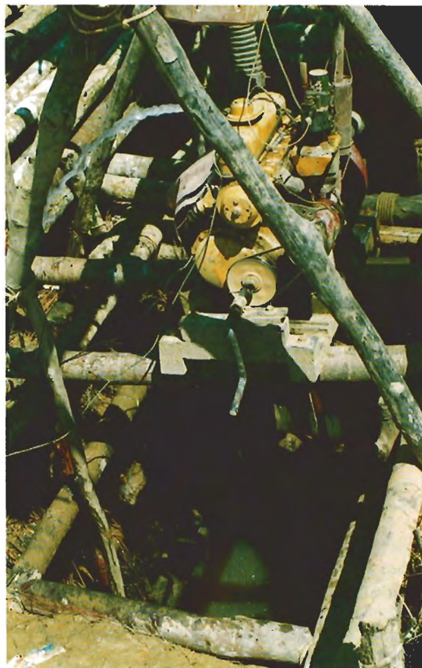
Figure 6. A car engine is commonly used to pump water from the mine shafts at Cempaka. Photo by David Dikinis.
