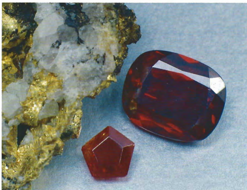
Figure 3. The red color of cuprite (the cushion cut) and cinnabar (the pentagon cut) has little to do with the fact that these gems contain copper and mercury, respectively. The color occurs because the band gap of these minerals is within the visible range: All wavelengths from violet to orange are absorbed, so that only red light is transmitted. The band gap in gold is much smaller than the energy of the visible range: All visible light is absorbed but some wavelengths are re-emitted preferentially, giving gold its yellow color and metallic luster. (Remember that the energy scale is inverse to the wavelength scale.) Photo by Robert Weldon.
