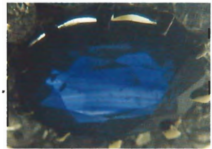
Figure 16. Two sets of curved color bands intersect in the wedge-shaped area at the center of this synthetic blue sapphire (7.5 x 5.0 x 3.1 mm). Magnified 10x.
