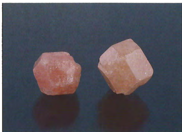
Figure 2. These two pink grossular crystals (12.07 and 18.35 ct) are from Xalostoc, Mexico. Their lack of spectral features distinguishes them from pink pyropes. Photo by Shane McClure.
