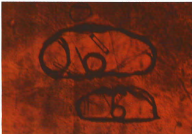
Figure 1. Three-phase—solid, liquid, and gas— inclusions are readily visible in this yellow sapphire from Sri Lanka. Note in the top two photos how the gaseous bubble is able to move about the crystal without restriction. With gentle heating in an immersion liquid, the gas bubbles gradually decreased in volume until they were totally homogenized (bottom right), at which point the temperature of the immersion liquid was measured in an attempt to verify the identity of the gas. The transparent, needle-like to tabular mineral inclusions are attached to the walls of the negative crystals. Magnified 65×.
