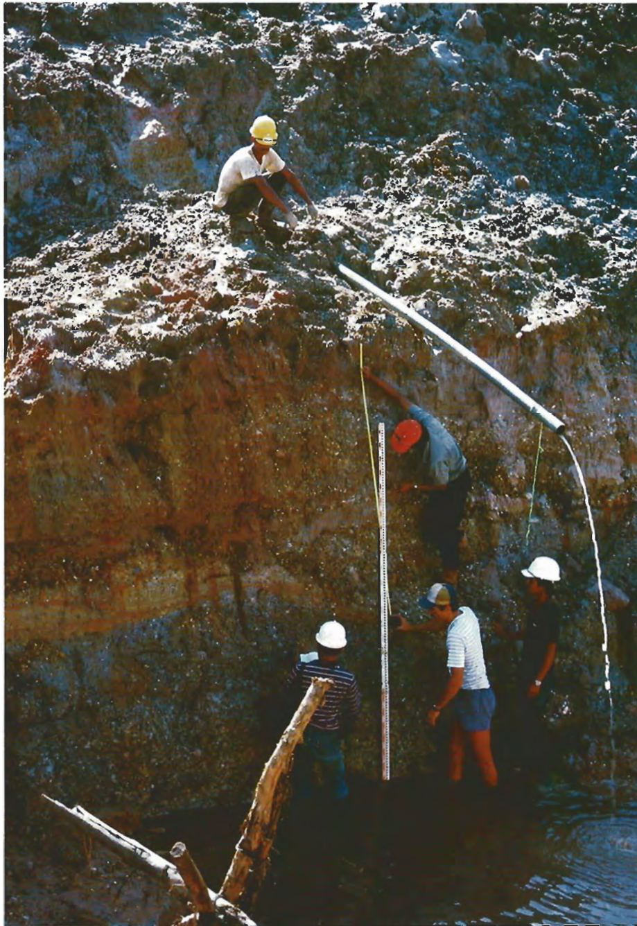
Figure 4. In this view of the wall of one of the sample pits dug by Acorn Securities at the Danau Seran swamp, the upper alluvial gravels (the yellowish brown sediments that are the principal source of diamonds) can be seen lying above the basal alluvial layer. Gravel thicknesses were measured at 1-m intervals all around the inside walls of the pit. Photo courtesy of Acorn Securities.
