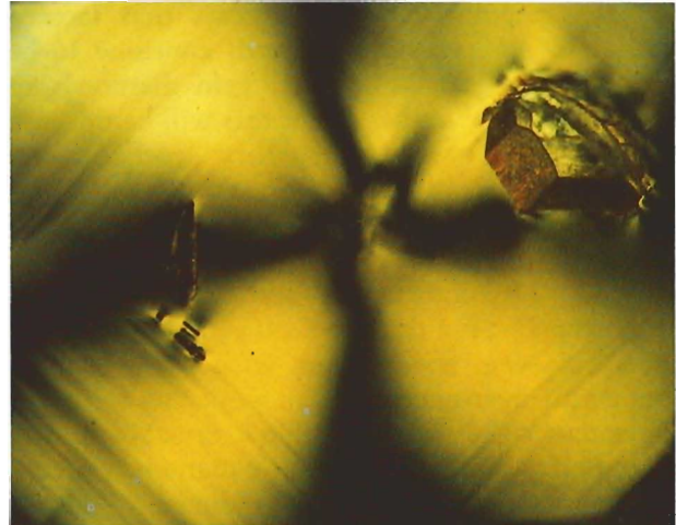
Figure 23. This cross-shaped internal strain pattern, here seen in a crystal, is distinctive of many of the De Beers synthetic diamonds. Note also the pattern of graining in the four cubic sectors. Cross polarized light; magnified 10 \times .
