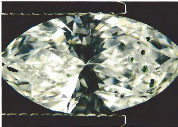
Figure 3. Bright green crystals of unknown identity are easily seen in this diamond. Magnified 10 \times .
