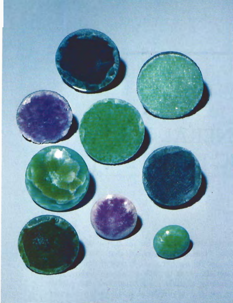
Figure 1. These nine synthetic jadeites manufactured by the General Electric Company were examined by the authors. The sample numbers of the jadeites, starting at the top row and proceeding left to right, are as follows: 7, 6; 9, 3, 1; 4, 8, 5; 2. The pieces range from 0.68 ct to 2.46 ct in weight. Photo © Tino Hammid.
