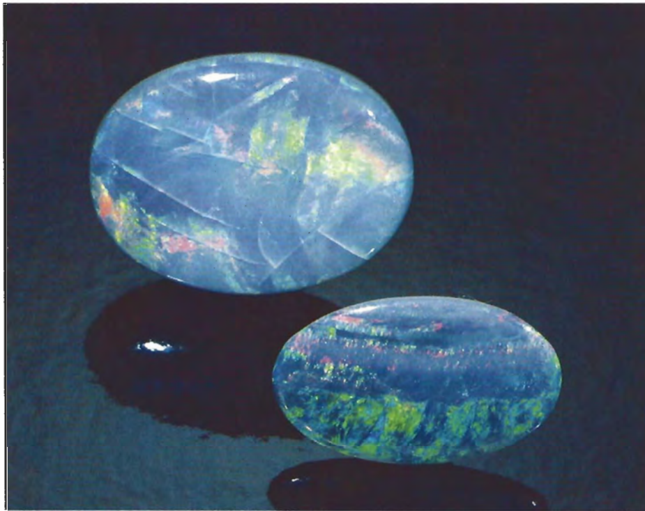
Figure 1. One of these two opals (7.00 and 1.14 ct) has been treated with polymer to improve its play of color, while the other is completely natural. No traditional gemological tests can distinguish between the two and, until now, laboratory testing took hours. With the infrared techniques described in this article, however, identification can be done in a matter of minutes (see figures 6 and 8). Photo © Tino Hammid.
