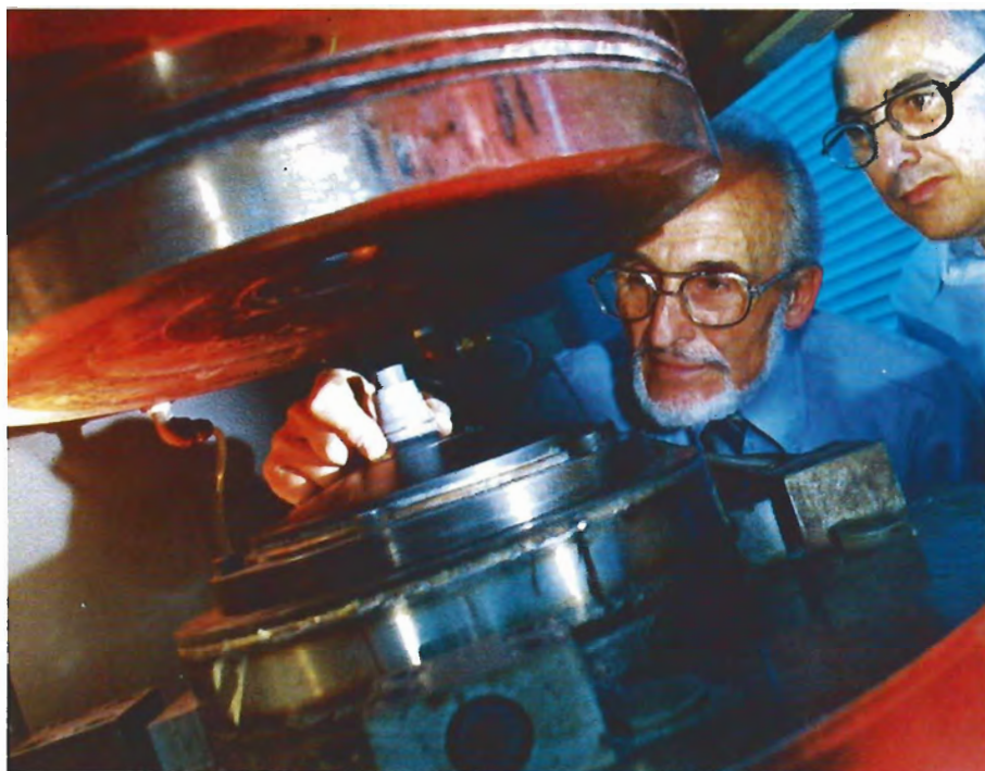
Figure 3. In this photograph of the high-pressure apparatus used to synthesize jadeite, R.C. DeVries is loading a sample into the apparatus while J.F. Fleischer looks on. Photo courtesy of the General Electric Company.
