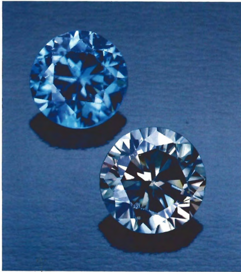
Figure 4. The grayish brown zircon on the right was the same color as the blue zircon on the left before it was exposed to long-wave ultraviolet radiation for 20 minutes. Note the radical color change. The most intense color obtained by this process—a muddy brown—was impossible to photograph because the lights required caused the stone to gradually revert back to its original color. Photo © Tino Hammid.
