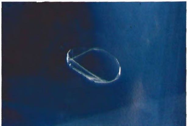
Figure 3. The same CO 2 -filled negative crystal as in figure 2 but just above the critical temperature (31.2°C) for carbon dioxide. Dark-field illumination, magnified 50×.
