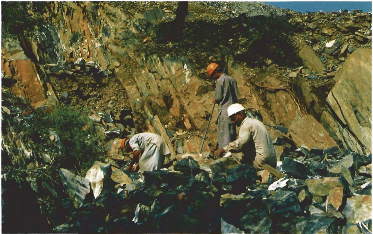
Figure 9. On a heap of blasted pieces of rock, miners break promising pieces in search of topaz crystals.
