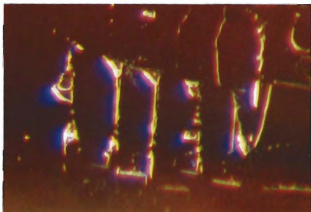
Figure 12. Discrete two-phase inclusions in parallel arrangement are commonly seen in pink topaz from the Ghundao hill, near Katlang, Pakistan. Magnified 50×.
