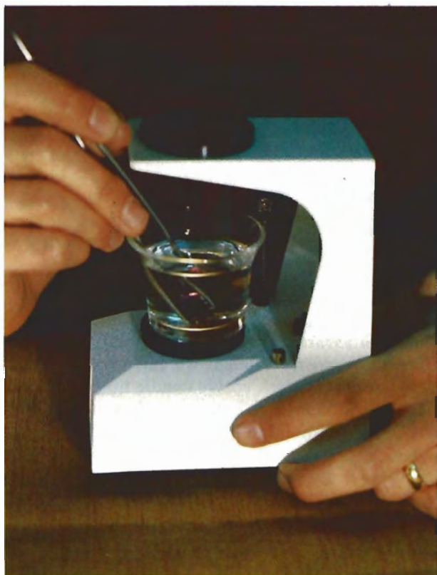
Figure 5. A simple polariscope and immersion cell are sufficient to identify Brazil twinning in near-flawless to flawless natural amethyst. Photo by David Hargett.
