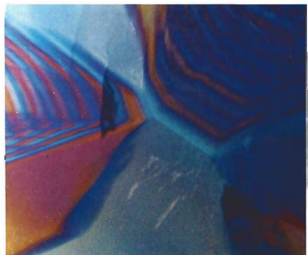
Figure 4. The twinning evident in this natural amethyst closely resembles the idealized drawing shown in figure 3. Note the narrow bands of color under the major rhombohedrons and the broad swaths of color under the minor rhombohedrons. Magnified 15x; photomicrograph by Robert Kane.
