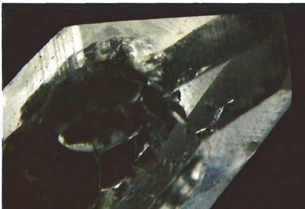
Figure 2. This colorless quartz crystal ( 18.1 \times 10.1 \times 7.3 mm) was core-drilled and filled with phosphorescent powder and epoxy resin. The piece was then capped to form a pendant.
