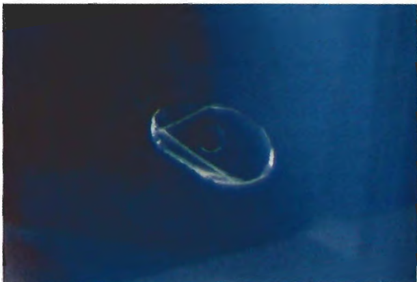
Figure 2. Negative crystal filled with liquid and gaseous carbon dioxide as observed below the critical temperature. Dark-field illumination, magnified 50×.
