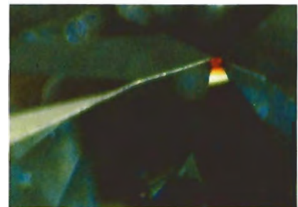
Figure 4. Irradiation stains on green diamond rough are sometimes altered to brown, as seen here, by the heat of polishing. Magnified 20×.
