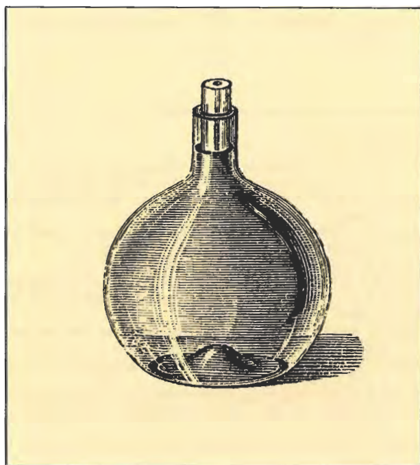
Figure 6. A pycnometer, or stoppered glass bottle, for determining specific gravity. From Groth (1887).
