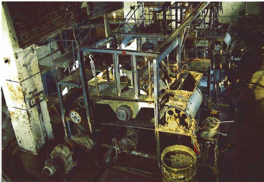
Figure 10. The final step in the recovery process is to pass the heavy concentrate over grease belts. Diamonds, being resistant to water, stick to the grease while other material passes over the belt. Periodically, the grease is scraped off and boiled to free the diamonds.
