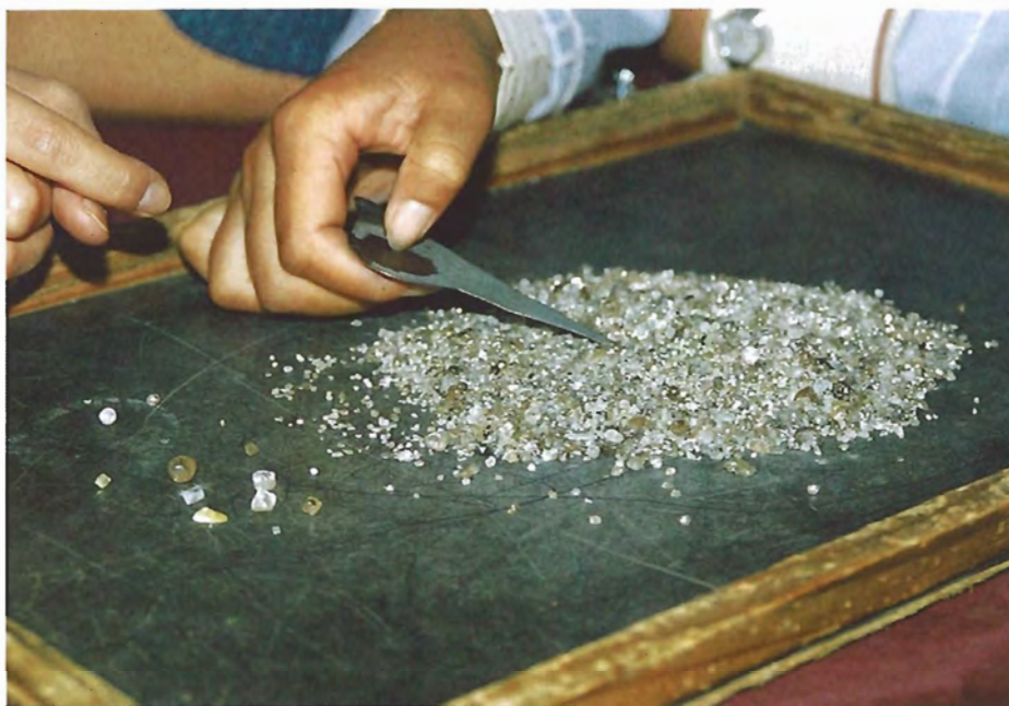
Figure 11. The diamond concentrate recovered from the boiled grease is sent to the sorting room, where any remaining kimberlite material is removed and the diamonds are separated into initial grades. The sample shown here is representative of mine-run diamonds from the Victory No. 1 pipe.
