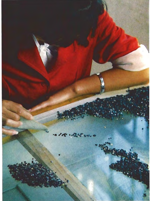
Figure 6. A glass table top lit from below is used to sort the gem crystals from the rest of the concentrate.
