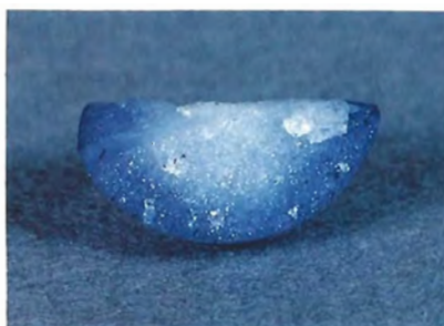
Figure 14. This broken portion of the imitation lapis lazuli bead in figure 13 shows the dye penetration into the quartzite.
