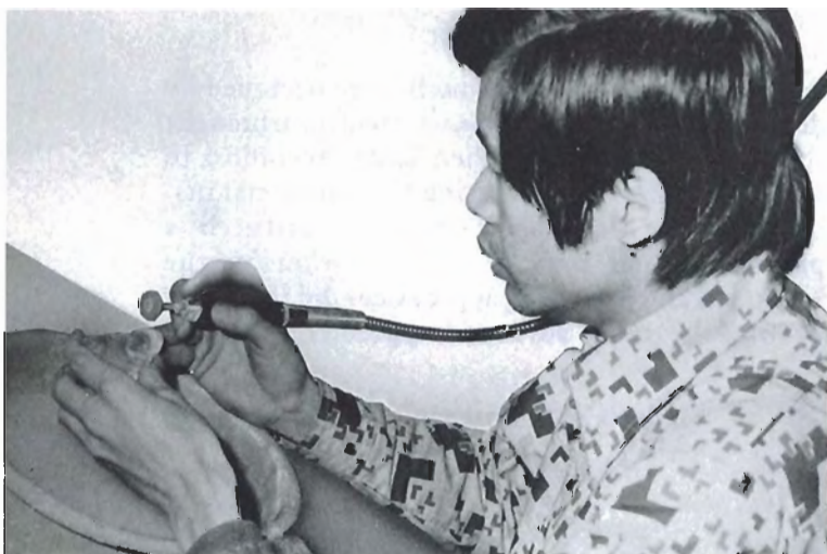
Figure 10. Modern Chinese power-driven carving machinery now uses diamond-impregnated tips instead of the traditional powdered abrasives.
