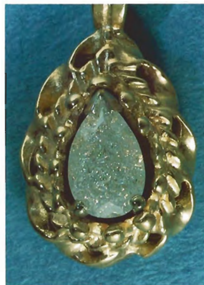
Figure 5. This 5.9 x 4.1 x 2.5-mm cubic zirconia was damaged by the heat of a torch while the mounting was being repaired.
