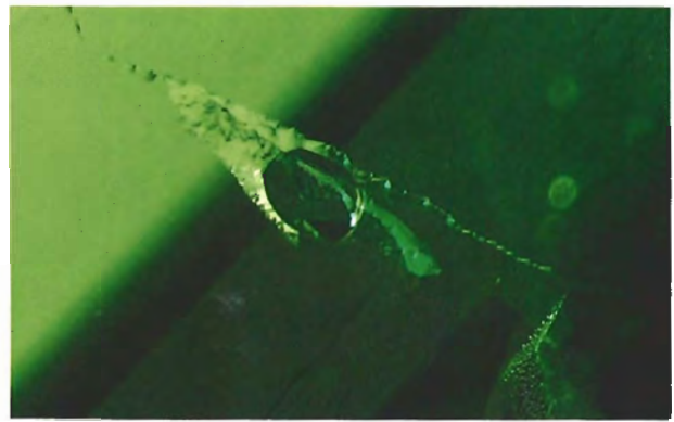
Figure 8. Captured within this Biron synthetic emerald is a large, well-formed, two-phase inclusion. Note also the fingerprint patterns at either end of the inclusion. Dark-field and oblique illumination, magnified 40 \times .
