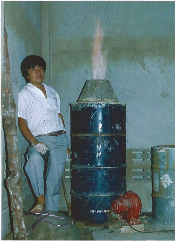
Figure 15. A Thai furnace typical of those used to treat rough Australian sapphire.
