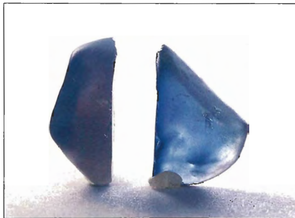
Figure 14. This single piece of Australian sapphire was cut in half and the piece on the right heat treated. Note that while there is improvement in clarity and color, the change caused by heat treatment is not as dramatic as that commonly seen in white or light-colored Sri Lankan sapphires that are turned blue by heat treatment. Photo © Tino Hammid.
