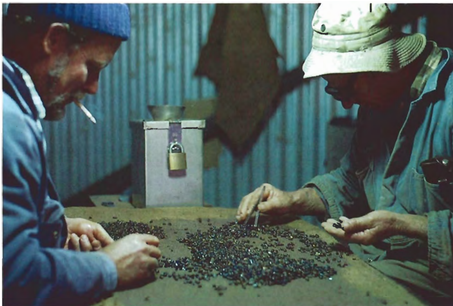
Figure 7. Picking out the sapphire from the coarse concentrate at an Inverell (New England fields) mine site.
