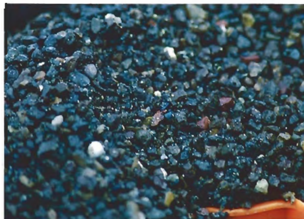
Figure 8. Fine concentrate after removal from the pulsator. Note the abundant black pleonaste.
