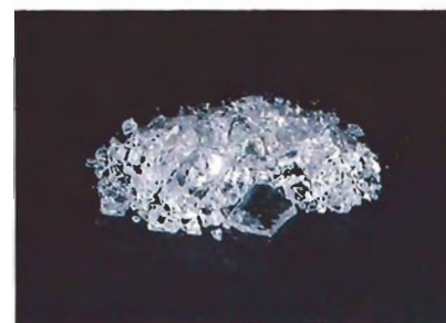
Figure 6. Remains of a strontium titanate after a torch was used to repair a piece of jewelry set with this diamond simulant.
