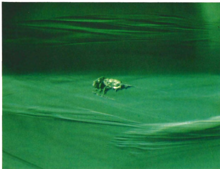
Figure 17. Several forms of growth features surrounding an unusual two-phase inclusion in a Biron synthetic emerald are accentuated by shadowing dark-field illumination. Magnified 40 \times .
