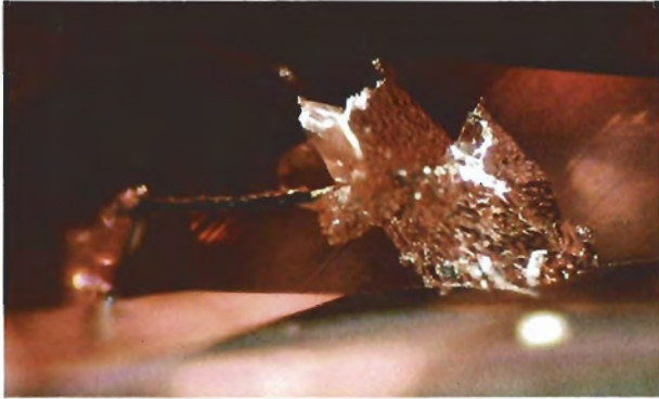
Figure 12. A part of the original surface on the girdle of this pink diamond shows evidence of "frosted" etching. Note the small amount of dirt or polishing material that has remained intact in the narrow section parallel to the girdle plane. Magnified 20x.
