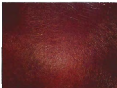
Figure 2. Coarse subsurface rutile needles in a 6-ct diffusion-treated synthetic star ruby. Diffused light, magnified 40x.
