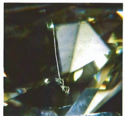
Figure 6. Step-like laser drill hole. Magnified 39 \times .
