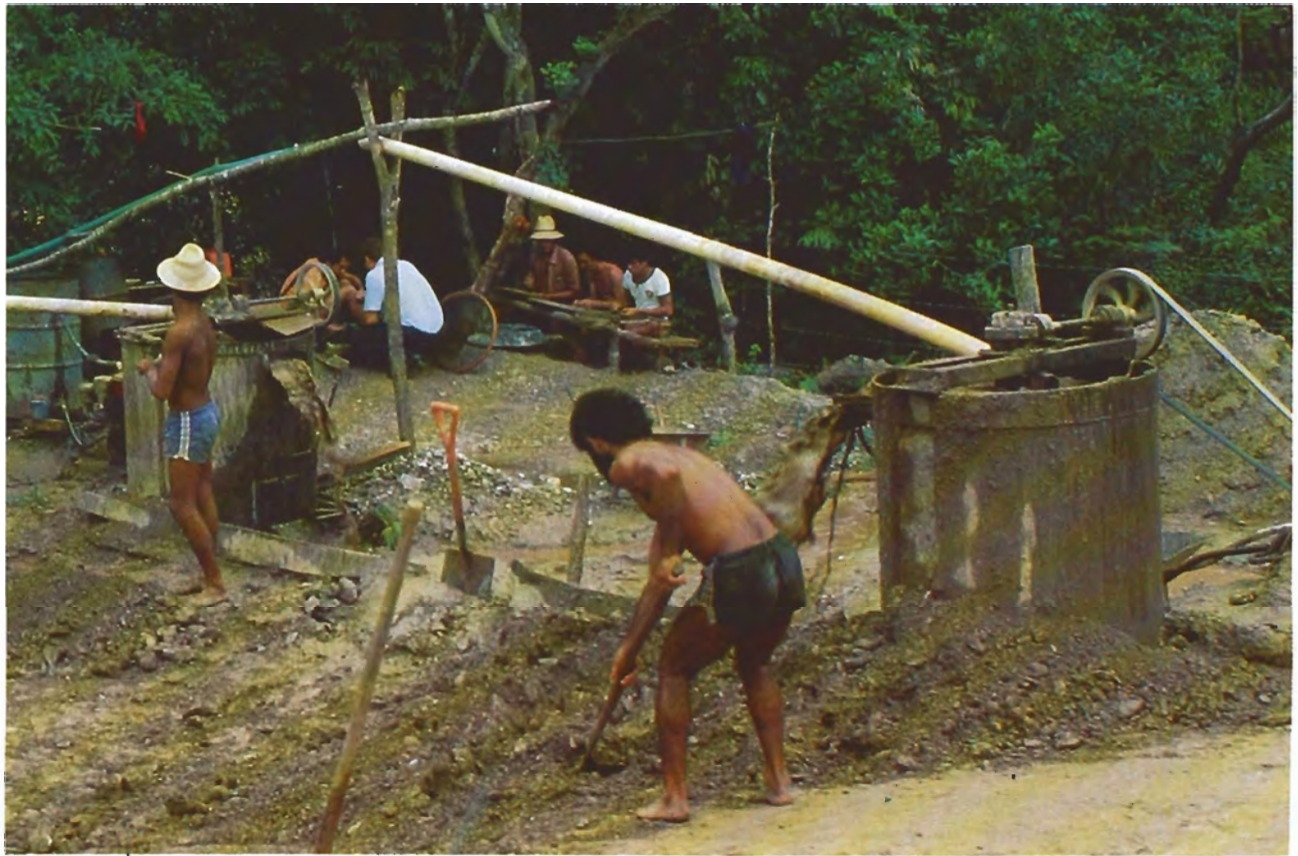
Figure 7. Ore is washed at Santa Terezinha de Goiás using large barrels, or "blenders," to separate the emerald crystals from the soft talc schist.
