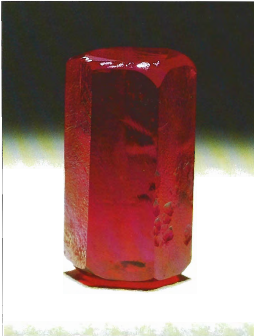
Figure 20. Synthetic ruby imitating a crystal, 10.96 \times 6.32 \times 5.10 mm. Notice the curved striae running vertically.
