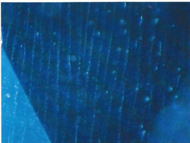
Figure 10. These stringers of minute gas bubbles are characteristic of flame-fusion synthetic spinel. Magnified 45 \times .
