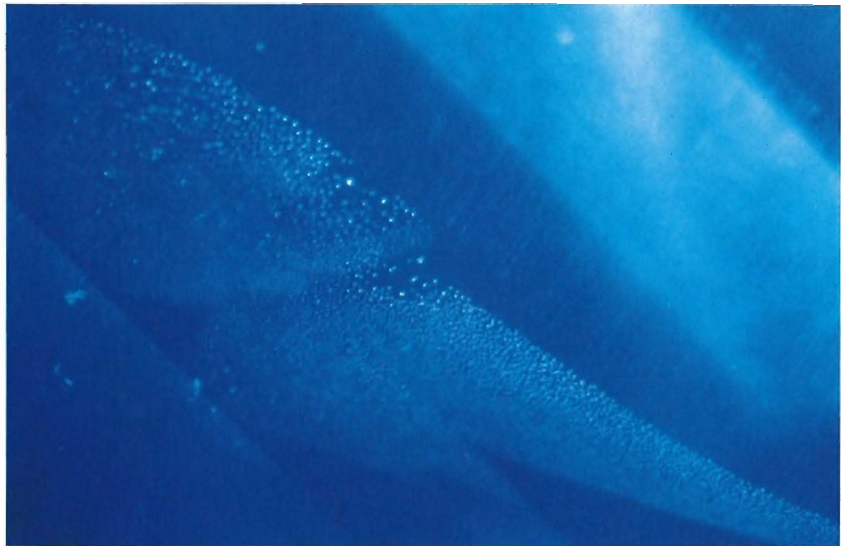
Figure 11. Borax (?) induced fingerprint in a flame-fusion synthetic sapphire. Dark-field and oblique illumination, magnified 65 \times .
