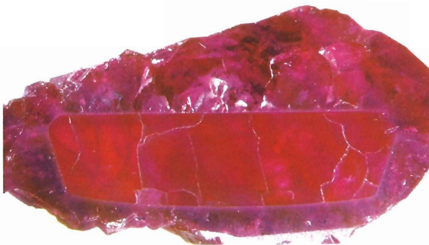
Figure 7. Cross-sectional view through the end of the experimental synthetic ruby illustrated in figure 6. Note the outline of the flux ruby layer over the flame-fusion core. Some fingerprints are visible even at this low magnification. Oblique and transmitted light, magnified 5×.
