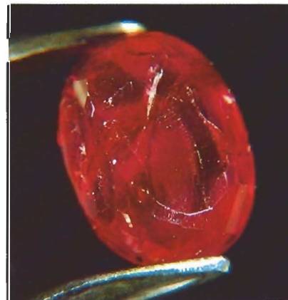
Figure 3. Note the internal fracturing and external chipping on this 2.55-ct ruby, caused by heat treatment. Magnified 16x.
