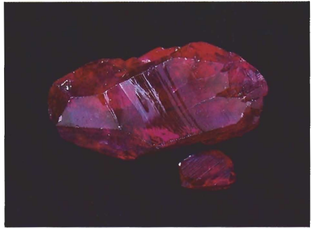
Figure 9. Two Verneuil flame-fusion ruby boule sections with a thin flux ruby overgrowth. Both of these samples contained numerous induced fingerprints. The largest sample is approximately 5 cm long. Photo by Mike Havstad.
