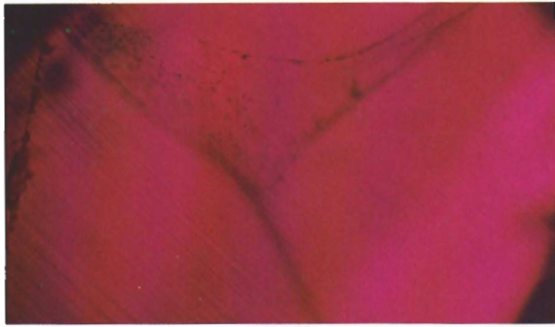
Figure 8. Induced flux fingerprint produced through experimentation in a Verneuil flame-fusion synthetic ruby together with the characteristic curved striae. Shadowing, magnified 45x.
