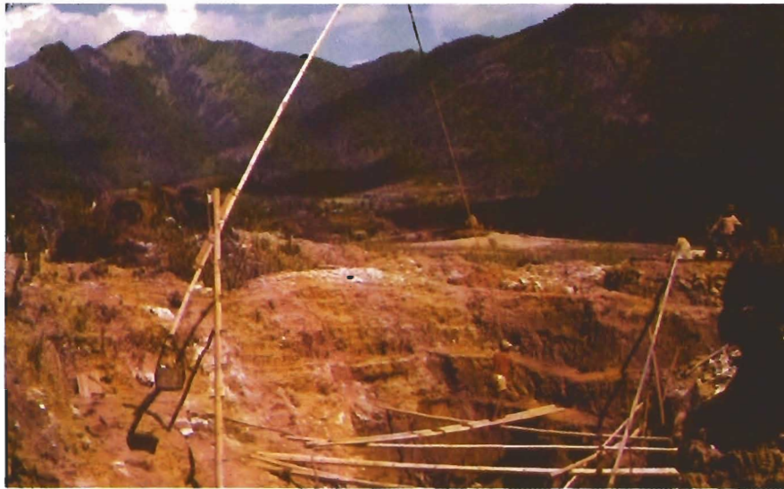
Figure 4. A twinlon, or circular pit, from which gem-bearing gravel is removed via the basket attached to the long bamboo crane shown here.
