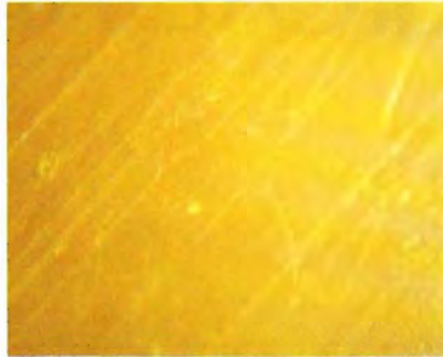
Figure 21. Striated structure of the surface of the bead-like core shown in figure 20. Magnified 63 \times .
