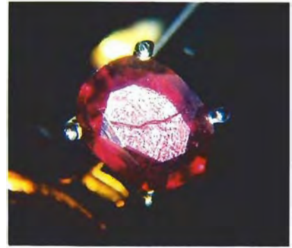
Figure 18. Reflection from the separation plane of a ruby and synthetic ruby assembled stone. Magnified 10×.
