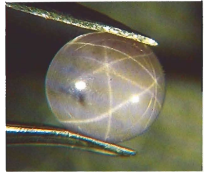
Figure 20. Four- and six-ray stars visible in the star spinel shown in figure 19.
