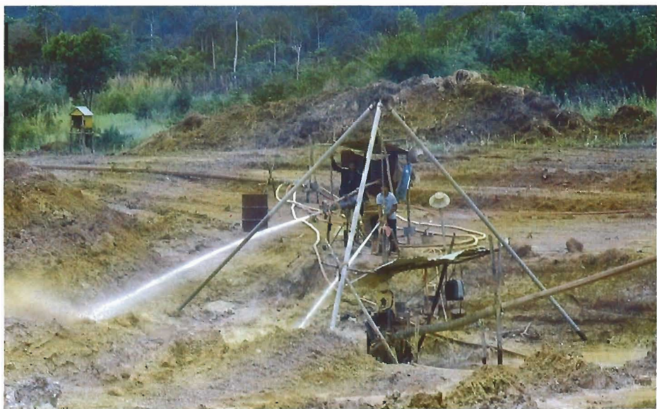
Figure 4. At Bo Rai, gem gravels are washed by high-pressure water cannons and transported up a pipe (seen to the right in photo) to a long sluice.
