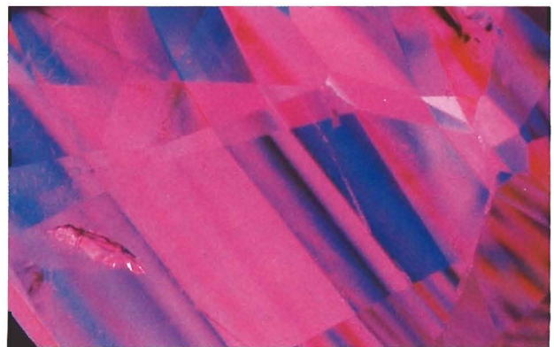
Figure 10. Polysynthetic twinning, here observed under crossed polarizers, is commonly seen in Thai rubies. Magnified 25×. Photo by John Koivula.
