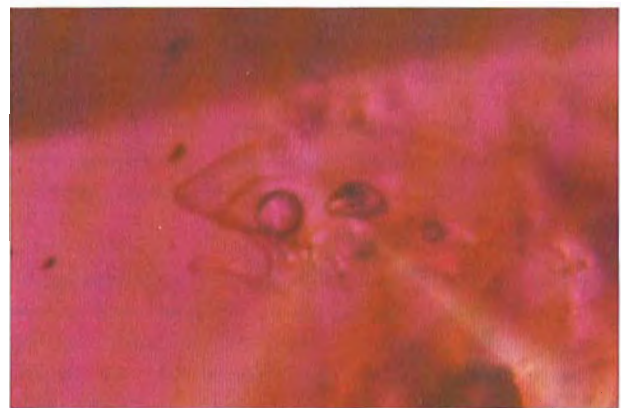
Figure 8. Complex underlaying of several two-phase inclusions with large gas bubbles and partly crystalline forms. Magnified 64 \times .
