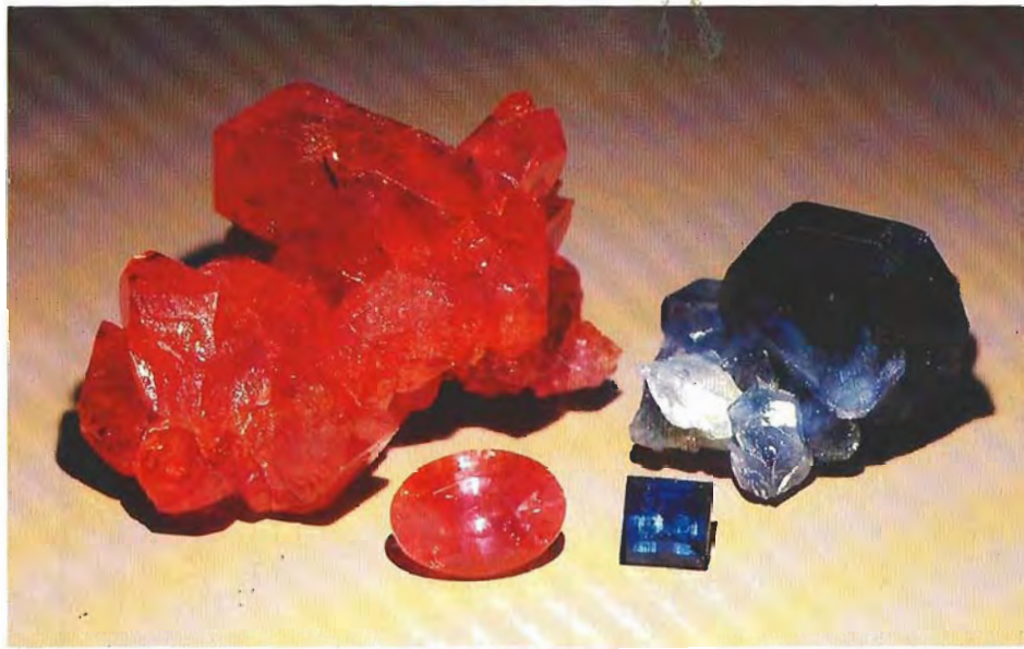
Figure 1. Exceptional examples of Chatham flux-grown synthetic orange sapphire (rough crystal group, 39.86 ct; faceted stone, 1.32 ct) and flux-grown synthetic blue sapphire (rough crystal group, 11.59 ct; faceted stone, 0.39 ct).
