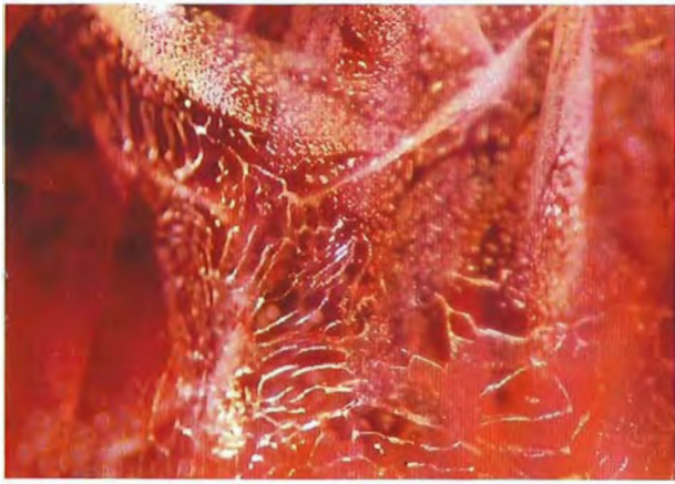
Figure 7. Transparent and nearly colorless, wide, mesh-like patterns of flux intersected by tightly arranged white "fingerprints" of flux in a Chatham flux-grown synthetic orange sapphire. Magnified 30 \times .
