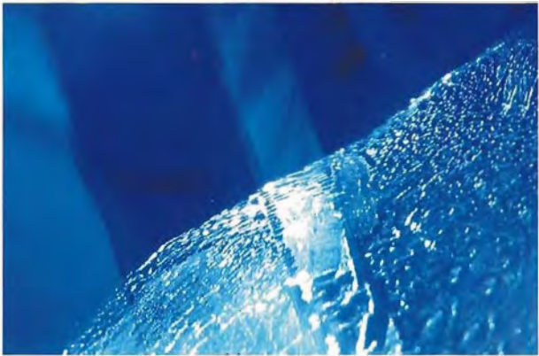
Figure 8. "Fingerprint" of white flux observed in high relief with straight-sided, angular, cloudy white zoning in a Chatham flux-grown blue sapphire. Magnified 25 \times .
