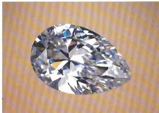
Figure 7. The Watermeyer split-facet pendeloque cut in cubic zirconia, 10.85 ct. Photo by Tino Hammid.
