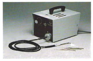
Figure 2. The quartz-halogen illuminator adapted for pinpoint illumination.
