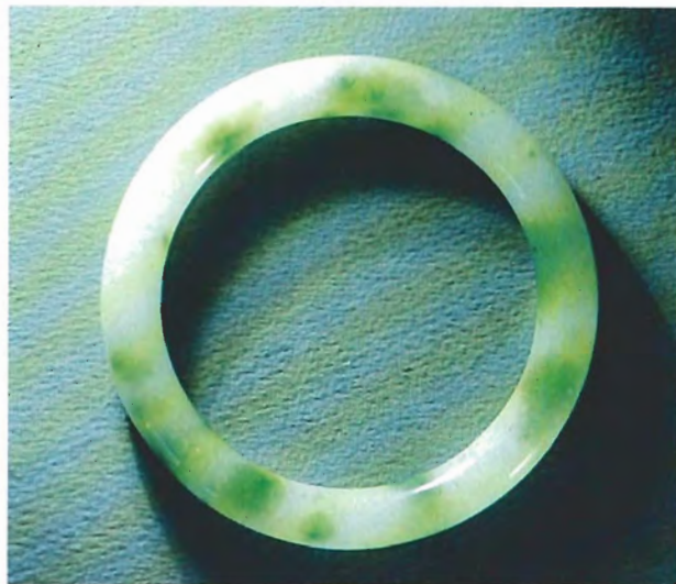
Figure 12. Dyed calcite such as this may look like jadeite, and its refractive index may be confused with that of jadeite. The birefringence blink technique is suggested for this material.
