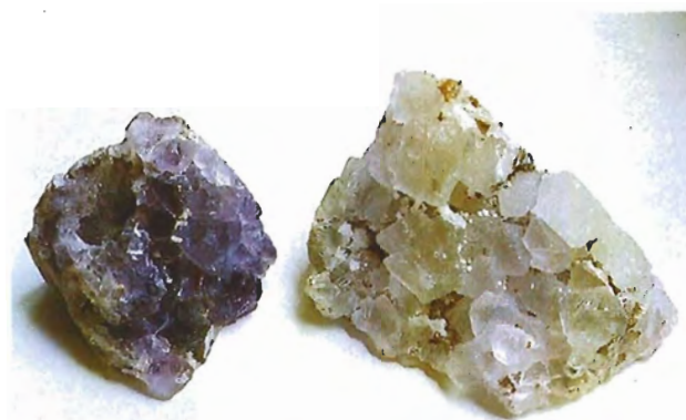
Figure 18. Fluorite before (colorless) and after irradiation.
