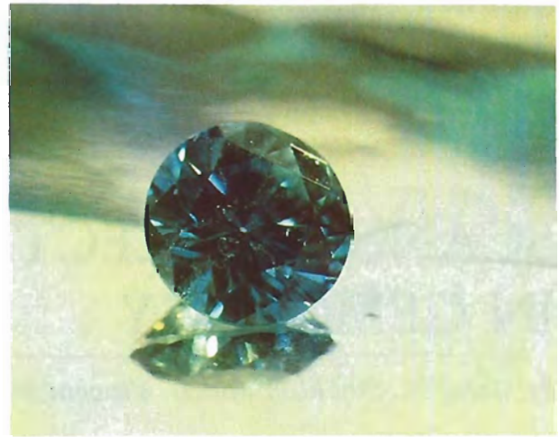
Figure 23. Diamond turned blue by electron-beam irradiation.
