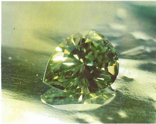
Figure 22. Diamond turned green by gamma-ray irradiation.
