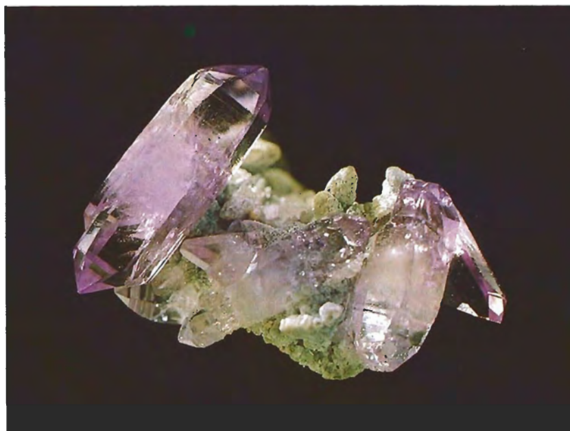
Figure 20. Amethyst color is the result of the irradiation (natural or artificial) of quartz that contains low concentrations of iron. This is a natural amethyst specimen from Vera Cruz, Mexico.
