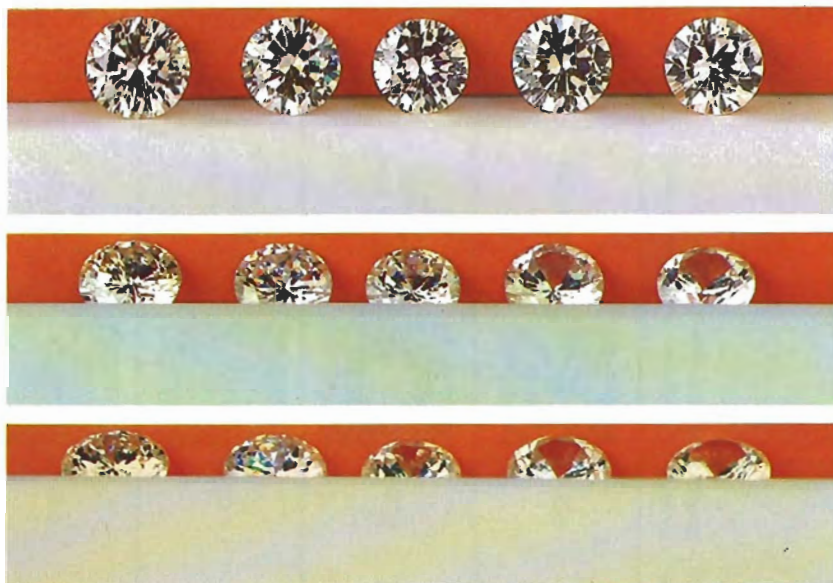
Figure 1. Diamond and its simulants will have different degrees of transparency, or read-through effect, if all are well-proportioned round brilliants. The lower the refractive index of the stone, the more obvious the read through is. Also, the greater the tilt, the clearer the read through is. Order from left to right (high to low R.I.): diamond, strontium titanate, CZ, GGG, YAG.
