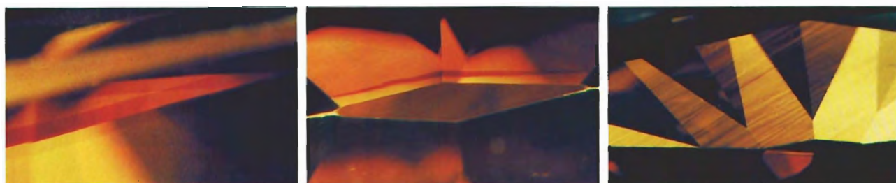
Figure 3. Cyclotron-treated diamond. Left = crown facets viewed through the pavilion, magnified 40 \times . Center = culet area viewed through the table, magnified 30 \times . Right = culet area and brown graining, magnified 12 \times .
