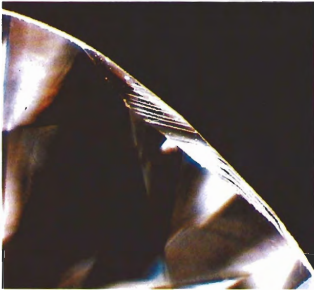
Figure 12. A natural, or part of the original crystal surface, is often found on or near the girdle of a diamond. Magnified 35 \times .
