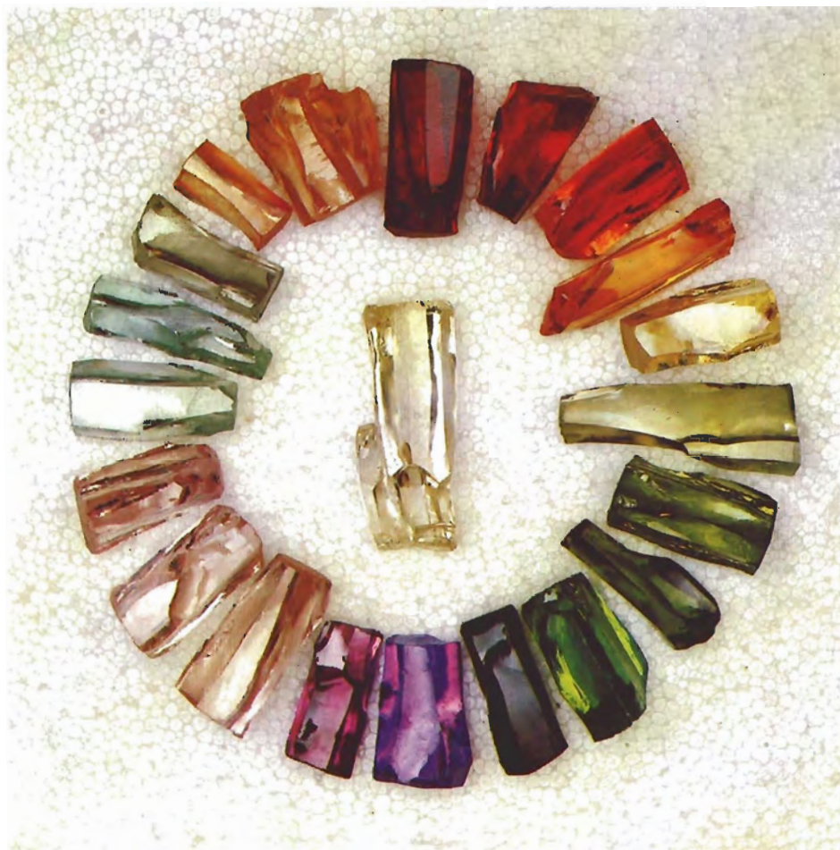
Figure 8. Colored cubic zirconia rough; the largest piece is 2.5 inches (6.5 cm) long. Courtesy of the Ceres Corp., Waltham, MA.
