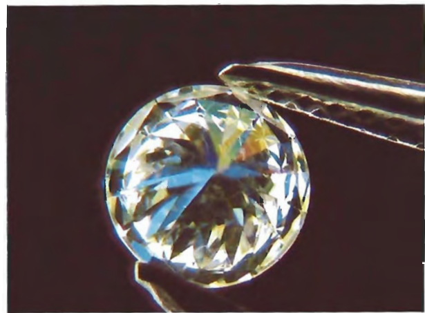
Figure 7. Dispersion: orange and blue extend over only a few facets of diamond. Magnified 10×.
