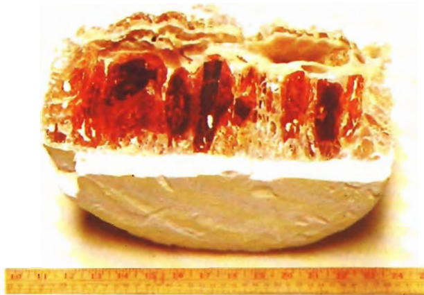
Figure 5. Half of a large skull of yellow cubic zirconia crystals grown using the technique described in figure 4. Courtesy of the Ceres Corp., Waltham, MA.
