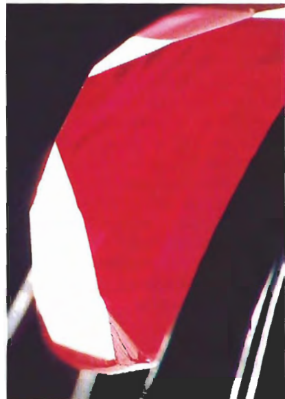
Figure 20. Angular banding in a flux-grown synthetic ruby. Magnified 30×.
