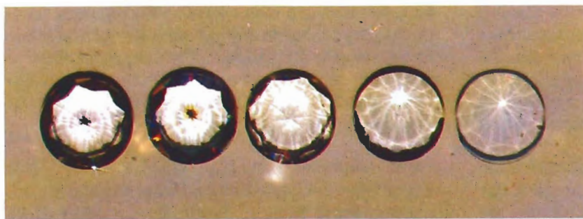
Figure 17. The higher the refractive index of the stone, the more distinct the stone is when immersed in methylene iodide and the darker and wider the shadow around the girdle is. Left to right (high to low R.I.): diamond, strontium titanate, CZ, GGG, YAG.
