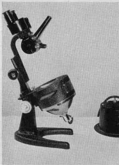
FIGURE 1 Diamondscope with Bausch and Lomb AK with Drum Nosepiece.
