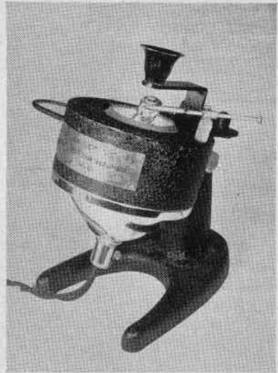
FIGURE 2 Diamond Imperfection Detector, with G.I.A. 10x Loupe.
