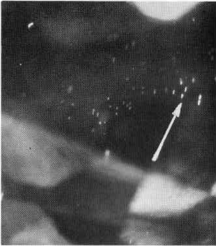
Figure 3. Colorless grossular with short stubby inclusions (60x). Arrow points to cluster of inclusions.
