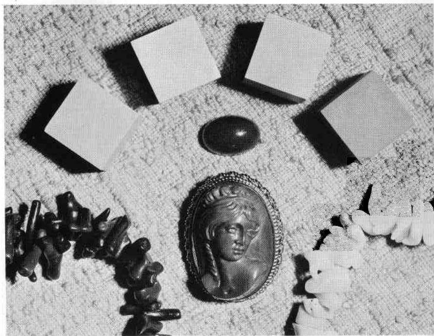
Figure 2. Four 14-mm cubes and one 10x14-mm cabochon of the Gilson "coral" with a natural coral cameo and two natural coral necklaces.
