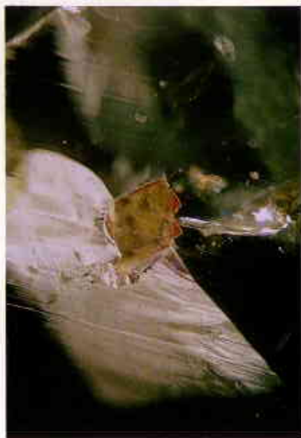
Figure 3. Yellow mineral inclusion of irregular shape, which the electron microprobe revealed to be a pyroxene. 100x
