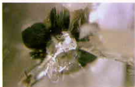
Figure 2. Common appearance of the black inclusions in the diamond slices examined. They usually consist of a central bright or black mineral surrounded by a system of divergent fractures. 100x
