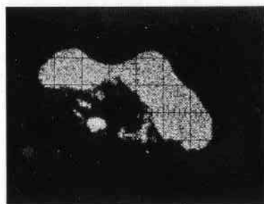
Figure 4d. Scanning X-ray image reveals that the copper content is mainly concentrated along the rim of the poly-mineralic grain of sulfides.
