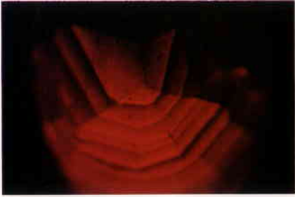
a. Synthetic alexandrite with growth banding showing changes in composition.
