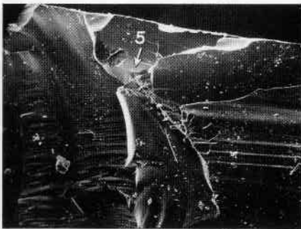
Figure 4. Photograph of a large fracture surface of the Slocum stone. (Photo taken with the Scanning Electron Microscope (SEM) at 53x.)
