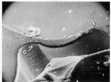
Figure 5. High magnification photo of the lenticular texture of the Slocum stone. (Photo taken with the Scanning Electron Microscope (SEM) at 680x.)
