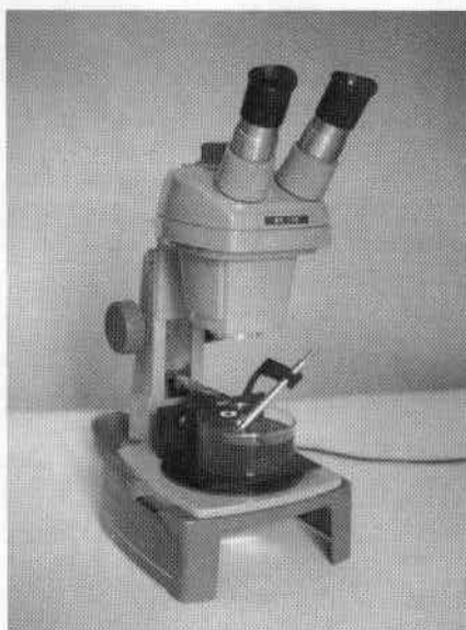
Figure 2. The crystal orienter on microscope stage with gemstone immersed in liquid and the accessory lens swung into position to observe interference figure.
