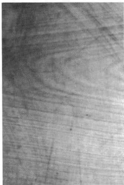
Photomicrograph of deer horn imitation of Hornbill ivory from India, showing concentric and orderly structure indicating growth. (30X.)
