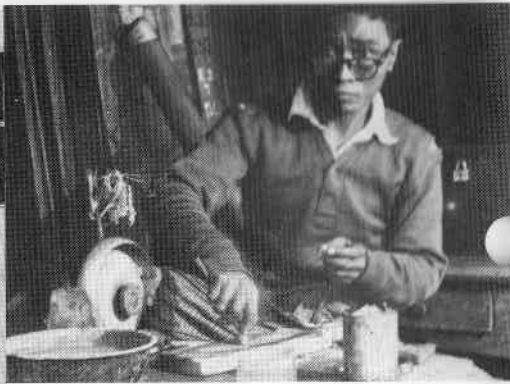
Figure 2 Jade lapidary, squatting behind a low bench polishes cabochons and buttons on a grooved board covered with Carborundum.
