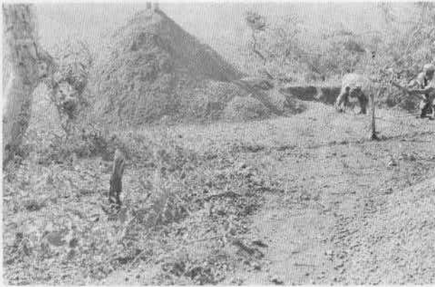
Alluvial patch on a hilltop. The garimpeiros prepare the gorgulho by screening out the oversize, before trucking it down to the riverside for washing.
