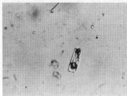
Figure 3. Strong magnification of pinpoint inclusions manifests them to be rectangular two-phase inclusions. (500x)
