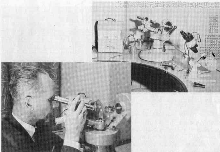
Dr. Edward Gubelin measuring the angles of a brilliant-cut diamond with the two-circle goniometer in his diamondroom.
