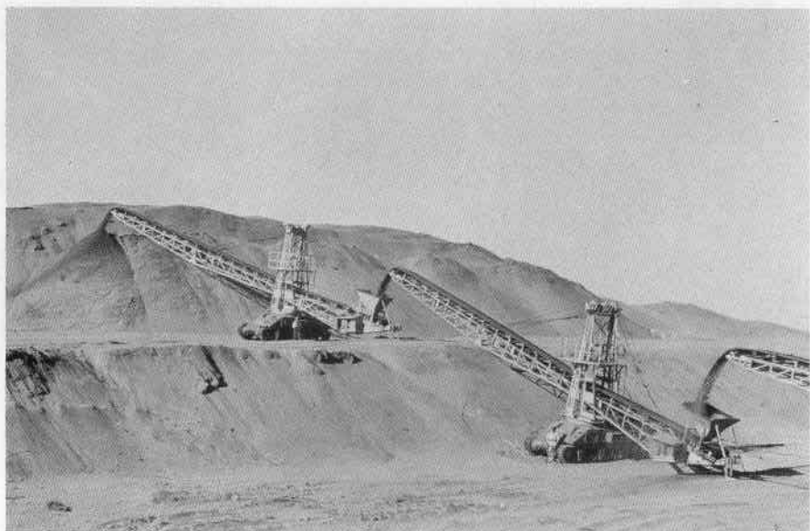
Portable stackers; note Sherman tank chassis
