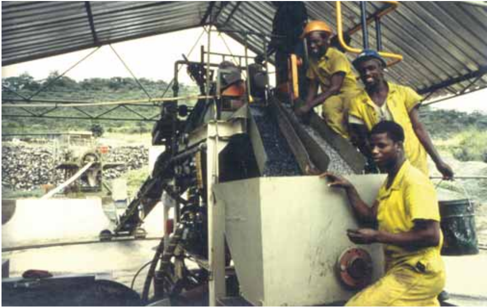
Fig. 30. The high-efficiency DMS (dense media separation) module is used at Sandawana to separate 'rich ore' (schist with emerald) from 'waste' material (usually pegmatite). A few hand-sorters are on the spot to 'save' the occasional emerald which occurs in the pegmatite.
