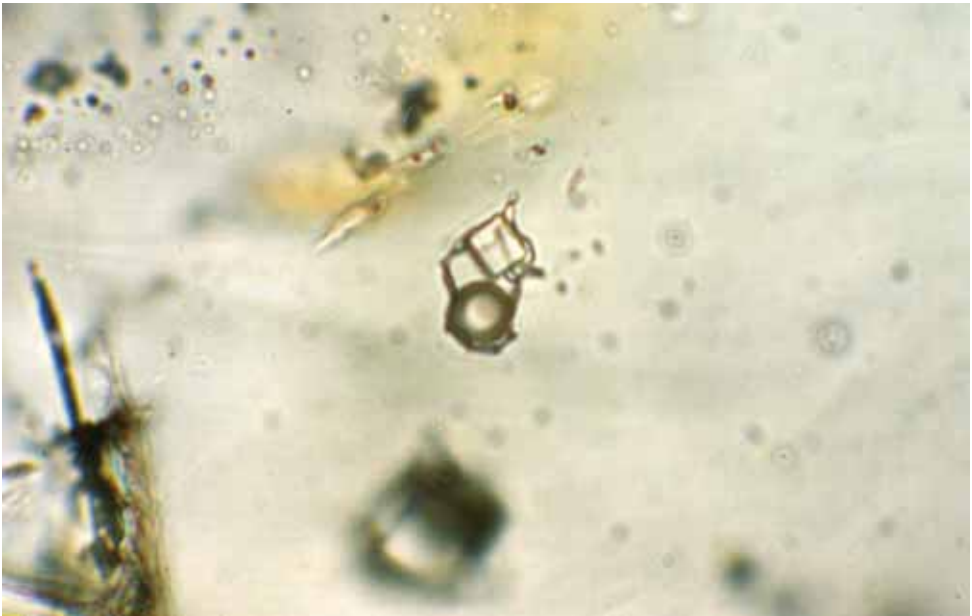
Fig. 60. Exceptional primary 3-phase brine inclusion found in emerald from Zeus 200ft level, 26/28 stope. Large halite cube, two small unknown solids, large dark gas bubble, containing traces of \text{CO}_2 , remaining fluid = saturated liquid water. Length of the inclusion is about 20 \mu\text{m} . (Width of view 120 \mu\text{m} ).
