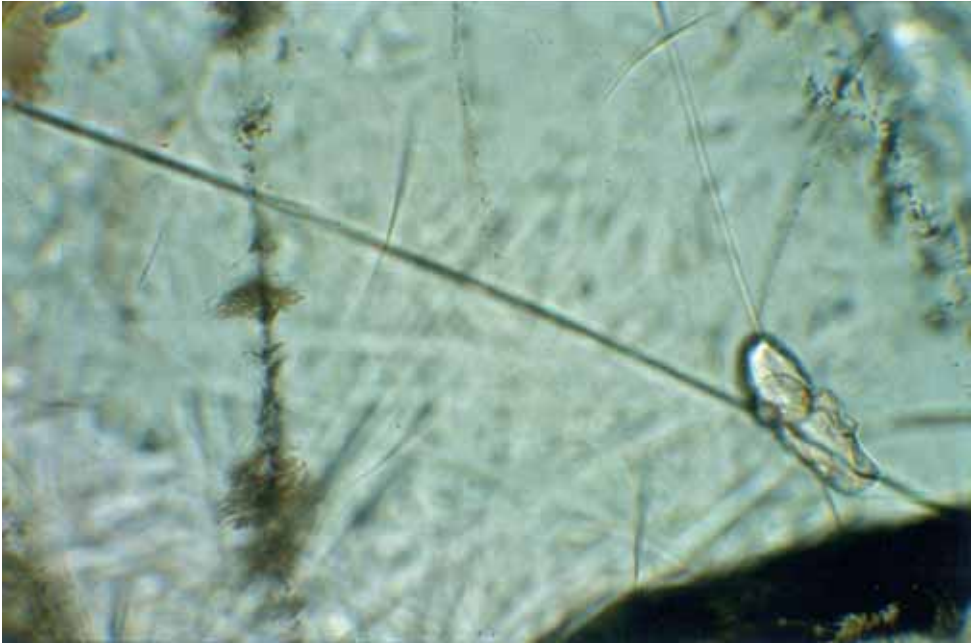
Fig. 59. The trail with decrepitated inclusions on the left is a common feature in Sandawana emeralds; it indicates the earlier presence of fluids. Albite crystals are visible on the right. Transmitted light, \times 125 .
