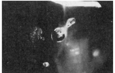
Figure 14.6 Circular stress flaw surrounding an inclusion which has expanded and turned white in a heat-treated geuda sapphire. (A. Good)
