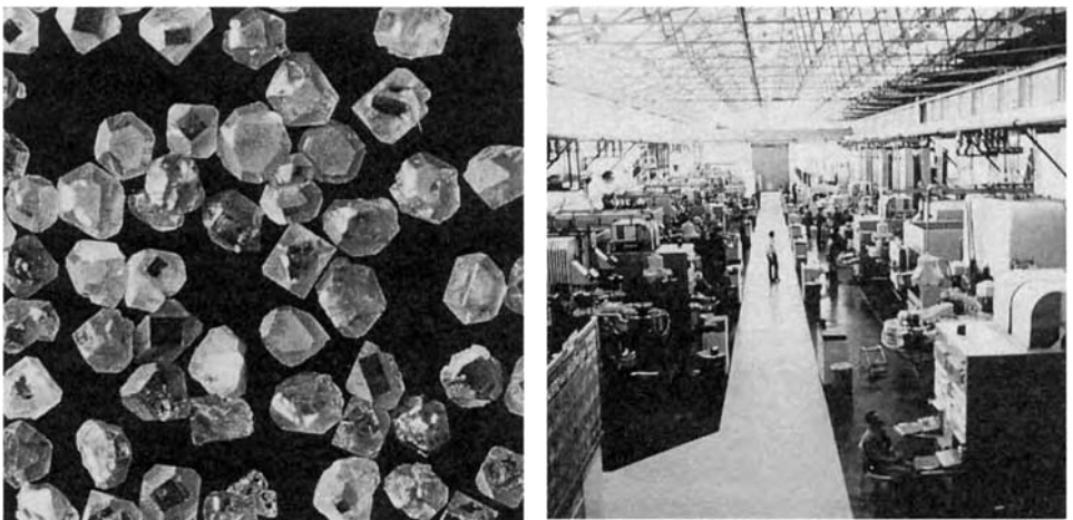
Figure 15.14 (left) Very small blocky crystals of synthetic industrial diamond. The habit of the crystals can be modified by adjustment of the process temperature and pressure. (right) A production unit containing a group of high-pressure presses used in the De Beers synthetic industrial diamond process. (De Beers)
