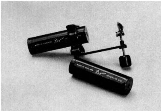
Figure 10.9 Two calcite dichroscopes. The one at the rear is fitted with a rotatable gemstone mount. (Gem-A Instruments Ltd)
