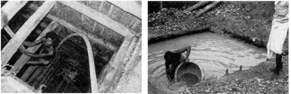
Figure 2.7 (left) Gem mining near Ratnapura, Sri Lanka – a shaft sunk to recover the layers of alluvial gem gravel: (right) Using a woven basket to wash and concentrate the recovered gem gravels
