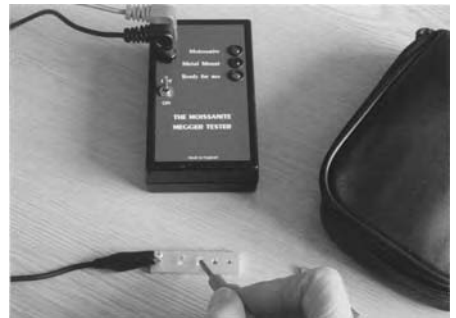
Figure 12.8 (left) A test circuit for checking the electrical conductivity of gemstones. (right) The battery-operated Synthetic Moissanite Megger Tester Mk II detects the semiconductor property of this diamond simulant (see text). The tester also verifies the semiconductor property of natural blue diamonds and synthetic boron-doped blue diamonds (diamonds whose blue colour has been artificially induced by atomic irradiation are non-conductors of electricity). (Gemmological Instruments)
