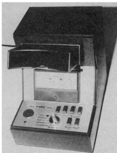
Figure 12.7 The Culti 'Color Stone Checker' contained both a LW and a SW UV lamp as well as a reflectance meter. The SW UV lamp was also used to check the transparency of gemstones at this wavelength
