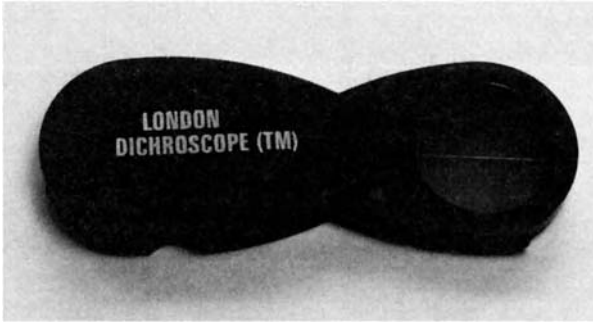
Figure 10.12 A dichroscope using a polarizing filter. The filter consists of two sections joined side-by-side, with the polarizing plane of one section rotated by 90^\circ to the other. (Gem-A Instruments Ltd)
