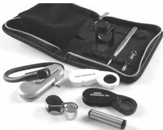
Figure 20.1 Gem-A Instruments Ltd standard gem kit consists of an 18 mm 10× hand lens, stainless steel tweezers, a folding polariscope with conoscope rod, Chelsea filter, Polaroid dichroscope, diffraction spectroscope, flexi torch, and a folding zip travel case. Gem-A Instruments Ltd professional gem kit has in addition a refractometer, a LW UV key ring, and an Osram flat light. The Polaroid dichroscope is replaced with a calcite version, and the hand lens and the spectroscope are replaced with wide-field versions
