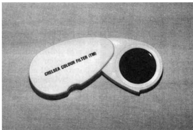
Figure 1.3 The Chelsea emerald filter designed to distinguish between emeralds and their simulants
