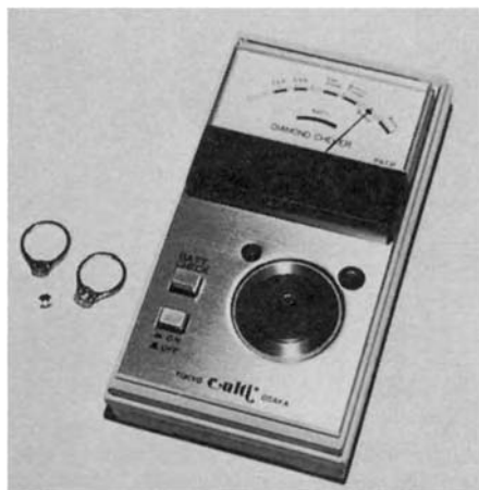
Figure 9.19 A single-range reflectance instrument whose meter is calibrated for diamond and its simulants. It uses pulse-coded infrared illumination and detection to minimize errors caused by ambient light
