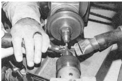
Figure 19.24 The bruter rondisting a sawn octahedral diamond. A corner of the other section of the sawn stone is clamped in a dop stick and used as the cutting tool. (Monnikendam)
