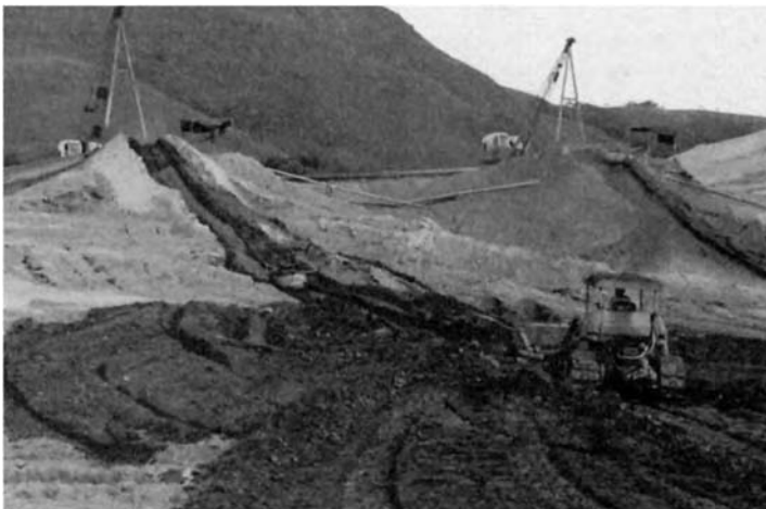
Figure 2.10 Drag-line removal of clay topsoil and excavation of gem deposits at the Capo do Lana topaz mine in Brazil
