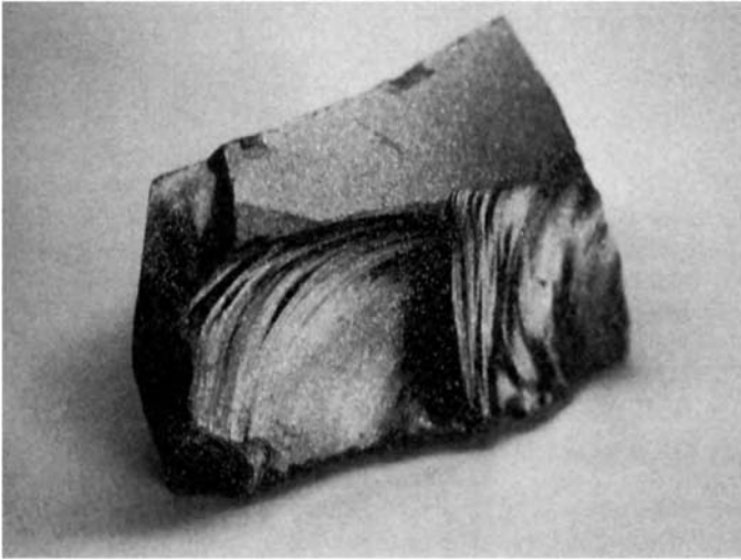
Figure 5.5 Conchoidal fracture in goldstone, a glass simulant of the feldspar gem sunstone
