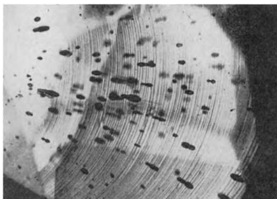
Figure 16.15 Curved growth lines and bubbles in synthetic Verneuil ruby
