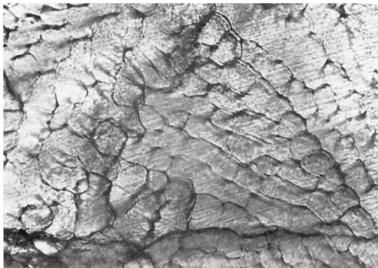
Figure 17.5 The 'lizard skin' effect seen in a Gilson imitation white opal
