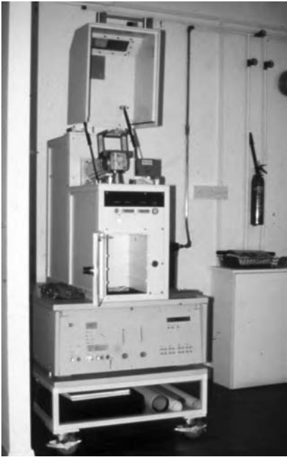
Figure 16.24 A specially commissioned X-ray unit used mainly for pearl testing (see pearl lauegrams in Chapter 18, Figures 18.11 and 18.12). (Courtesy of the Gem Testing Laboratory of Great Britain)
