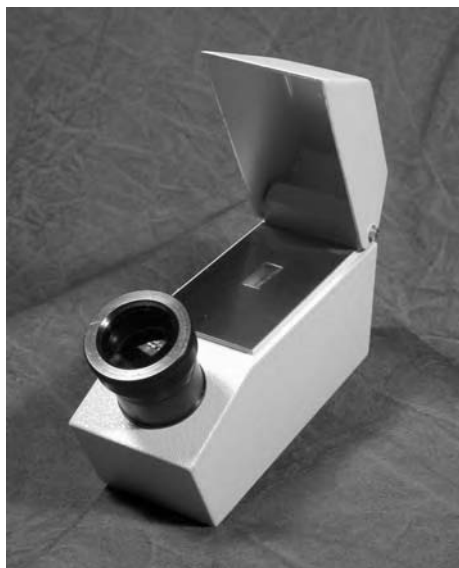
Figure 9.4 A typical critical angle refractometer, complete with built-in monochromator filter. (Gem-A Instruments Ltd)
