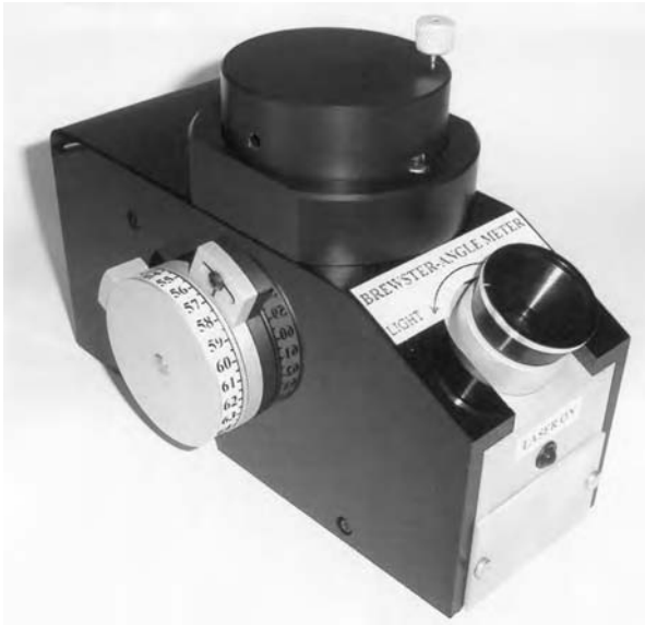
Figure 9.29 A Brewster-angle meter (developed by the author for Gem-A Instruments Ltd). The control is used to adjust the angle of the laser beam for minimum reflected light from the gemstone under test. The stone's Brewster angle is read from the control's scale and the gemstone identified from a set of tables.
