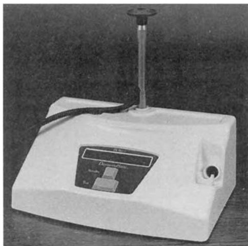
Figure 16.3 View of the De Beers DiamondSure (top) with its fibre-optic probe mounted vertically, ready to test the 415 nm absorption response of an unmounted diamond on the black test platform. When testing mounted diamonds, the test platform is removed and the tip of the probe is hand held against the diamond's table facet. The De Beers DiamondView (below) uses a video camera, placed vertically between two high-intensity SW UV light sources, and a specially configured computer/display (here showing an image of the fluorescent growth structure produced by a synthetic diamond). Special stone holders are available for unmounted and ring-set diamonds
