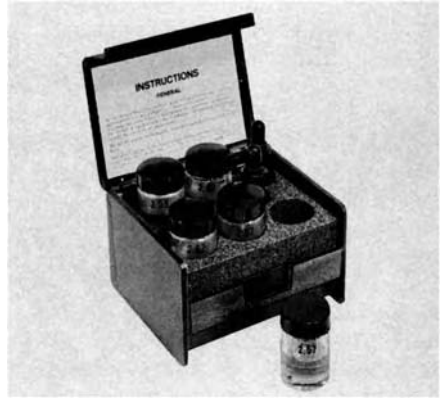
Figure 7.10 A set of five heavy liquids with two small bottles of adjusting fluids. (Kriiss)
