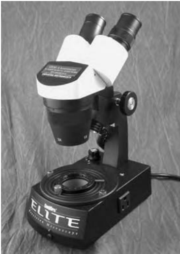
Figure 13.9 A low-cost stereo microscope using a turret lens system for 10 \times and 30 \times magnification using 10 \times eyepieces, a range which can be doubled with 20 \times eyepieces. (Gem-A Instruments Ltd)
