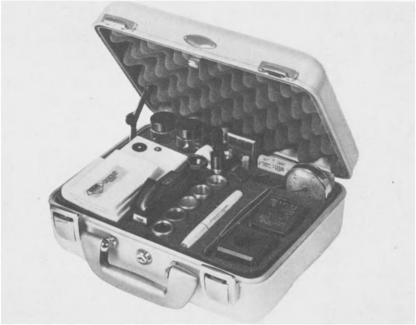
Figure 16.7 The Gem Maxi-Lab contains a full-size microscope as well as grading and identification instruments (Gem Instruments Corporation)
