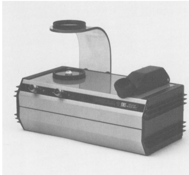
Figure 5.10 The Modul 1 unit is a combined refractometer and polariscope unit. (Eickhorst)
