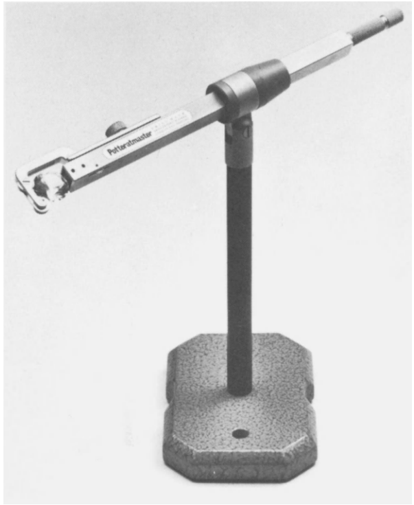
Figure 2.7 The Rayner stone holder uses spring-loaded jaws. If the base is removed the holder can be plugged into the clip hole on a microscope stage (Gemmological Instruments Ltd)
