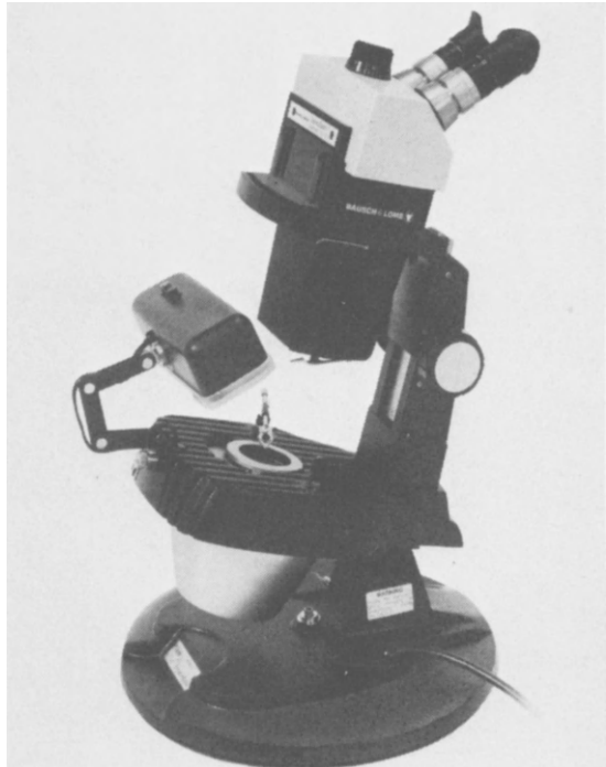
Figure 3.10 The Ultima B Mk V Gemolite (Gem Instruments Corporation)
