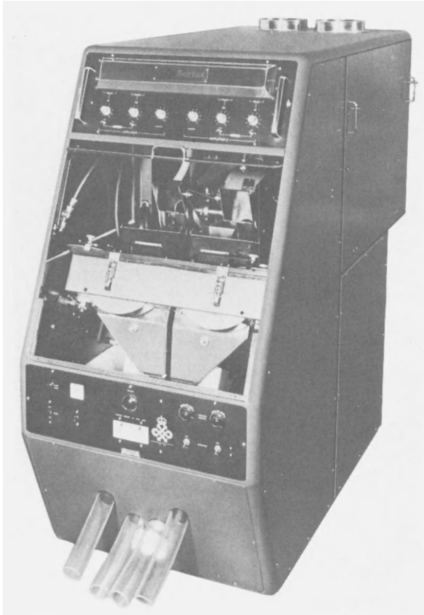
Figure 14.3 The Gunson twin-channel diamond colour sorter (Gunson's Sortex)
