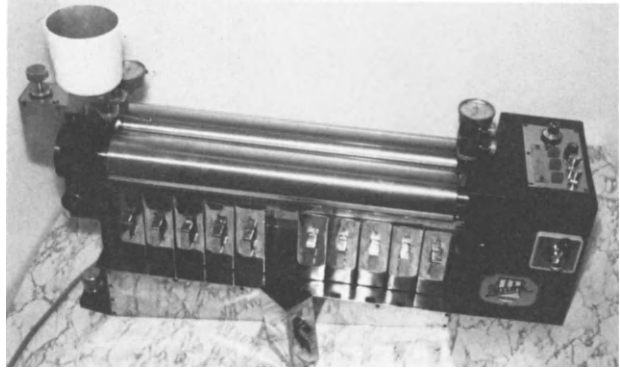
Figure 14.4 The Hauni roller sorter for separating diamonds by minimum diameter or thickness
