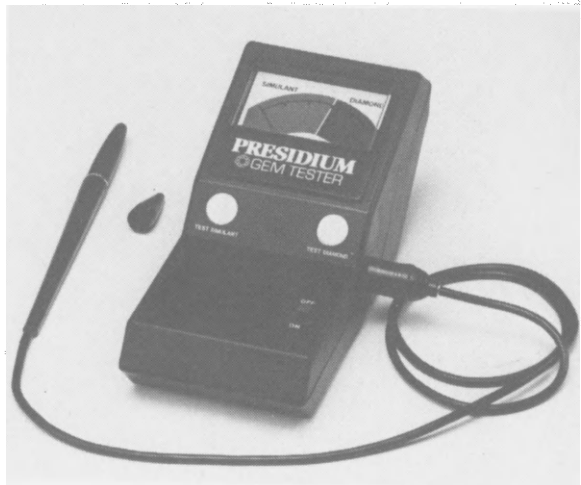
Figure 11.6 The Presidium Gem Tester is a portable unit employing a copper-constantin thermocouple probe
