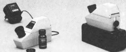
GemLED Refract. & built-in 589 nm LED Illum.
