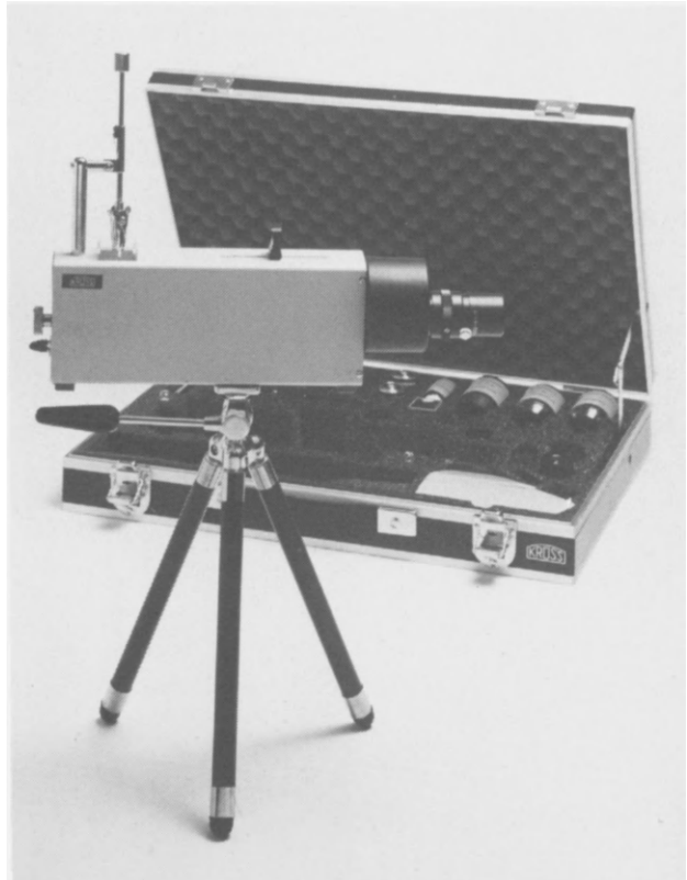
Figure 3.13 Portable microscope KA-4 as supplied with the portable laboratory KA-4KRS (Krüss)
