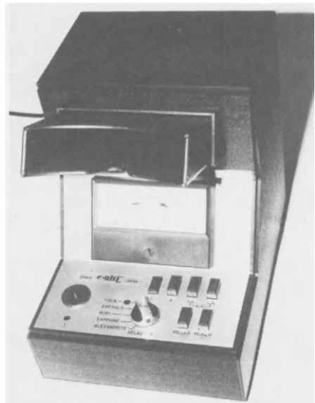
Figure 16.4 The Color Stone Checker contains a reflectivity meter, a LW/SW U-V unit and a U-V transparency tester (Culti)
