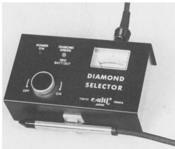
Figure 11.14 The Culti mains/battery diamond selector (Culti Corporation/Geshiro)
