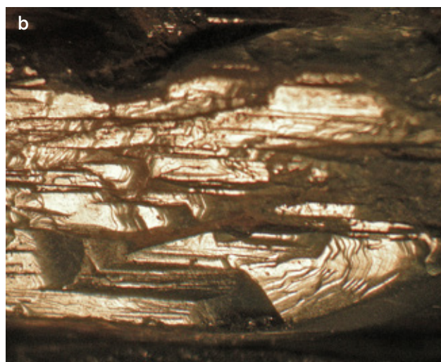
Figure 3: (a) Growth zoning in the Nigerian emerald (9.9 mm across) is visible in immersion in this view perpendicular to the c -axis, showing layers parallel to the basal pinacoid c and dipyramid p . (b) In reflected light, the prism faces of the crystal display grooves or surface indentations with a fine structure, as well as individual growth layers resembling contour lines on a topographic map (field of view 4.8 × 4.0 mm). Photomicrographs by K. Schmetzer.
