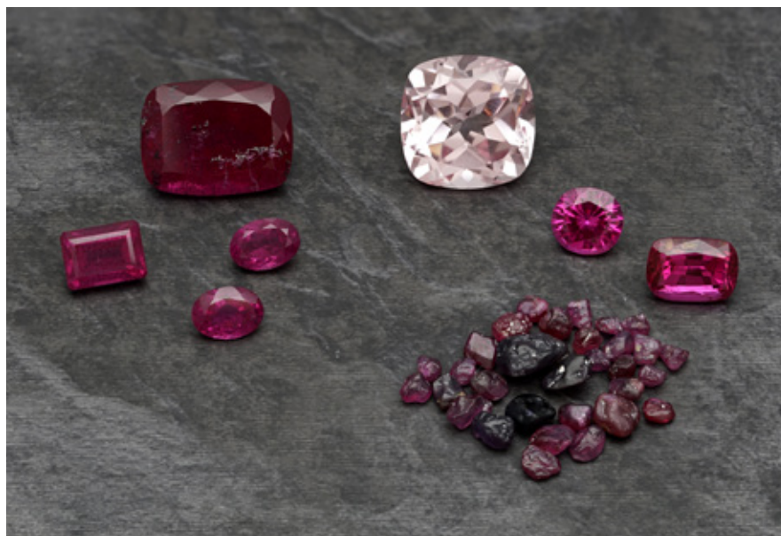
Figure 31: Five samples of synthetic corundum produced by the Kyropoulos method in Russia were examined for this study: four synthetic rubies (left) and a pink synthetic sapphire (top centre). For comparison, we also examined the two synthetic rubies on the right, which were produced in Idar-Oberstein by the Kyropoulos method in a modified Czochralski apparatus using natural rubies from East Africa (such as those at bottom right) as starting material. The faceted gems range from 1.52 to 18.69 ct. Photo by T. Stephan.
