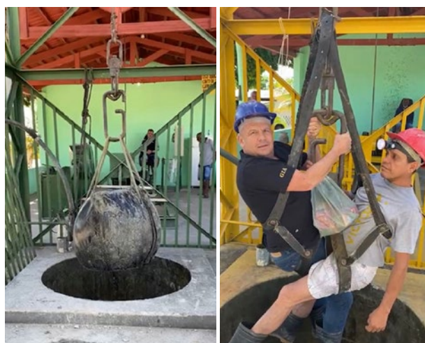
Figure 1: At the Lúvio Verde Mining joint venture, a winch is employed to transport the emerald-bearing talc schist to the surface in a large rubber container (left), and this system is also used in conjunction with a special harness to transport personnel in and out of the mine (right); the author is shown wearing a black shirt. Photos courtesy of M. C. Zenetos.
