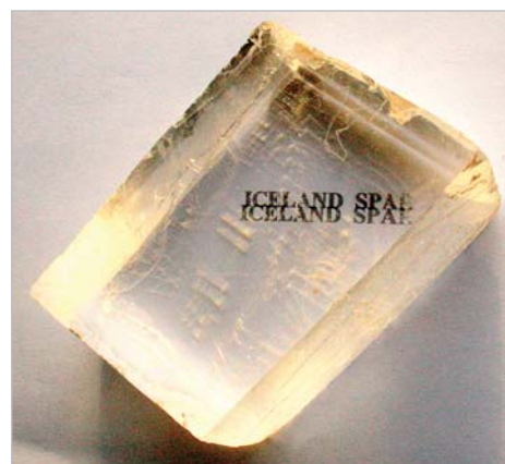
1: Double refraction by a rhombohedron of Iceland spar.
