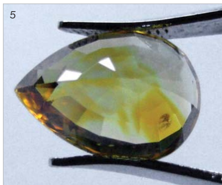
5: Although appearing even in colour when viewed from the table side, this 3.19 ct sapphire displayed strong colour zones when held up to a window and viewed through the pavilion.
