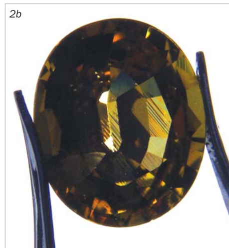
2: Yellow sapphire, 4.30 ct (a), when held up to light from a window, displayed internal straight graining (b).
