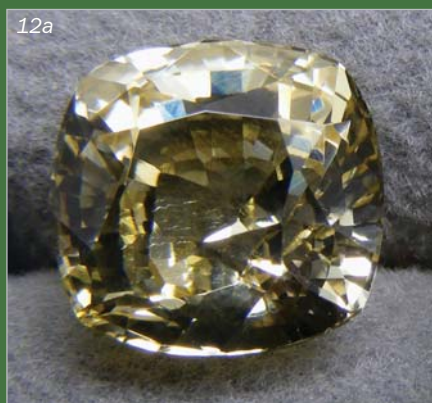
12(a and b): 'Fire-marks' on the pavilion facets of a 4.76 ct brownish yellow sapphire. Magnification (a) 8× and (b) 35×.
