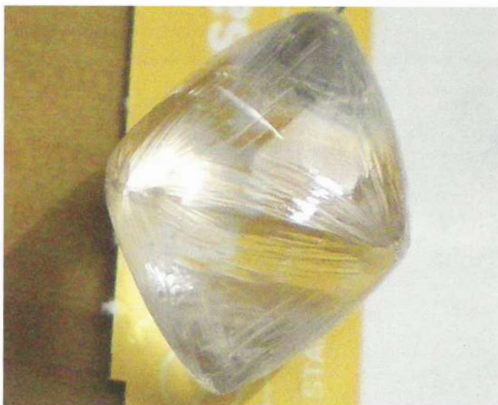
4: A perfect octahedron with an internal cleavage plane oriented NW-SE, not parallel to any of the octahedral faces, which are the cleavage directions in diamond.
