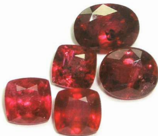
A selection of the glass-filled rubies recently acquired by the Gemmological Association for educational and research purposes. (See also Notes from the Lab, p.53)
