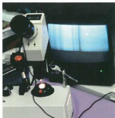
The Challenger spectroscope linked to a black-and-white TV monitor displays spectacular views of the absorption spectrum from 300 to 1000 nm from a standard diffraction spectroscope.
