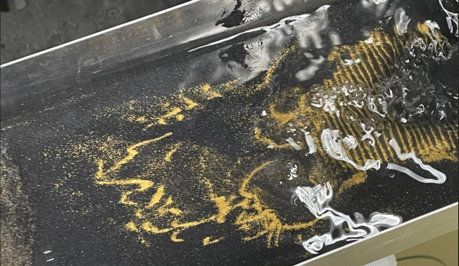
Flour gold captured in the magnet sluice. This is where the recovery of smeltable concentrates of tiny gold and gold ore occurs. Photo courtesy of John Schoonover.
