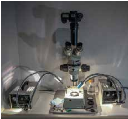
1. Left: The author's Nikon SMZ10 stereomicroscope with gemmological base and fibre-optic illumination setup. Right: The author's custom vintage Zeiss Universal compound microscope equipped with differential interference contrast (DIC) components, which facilitates the examination of surfaces of gem materials at high resolution.
