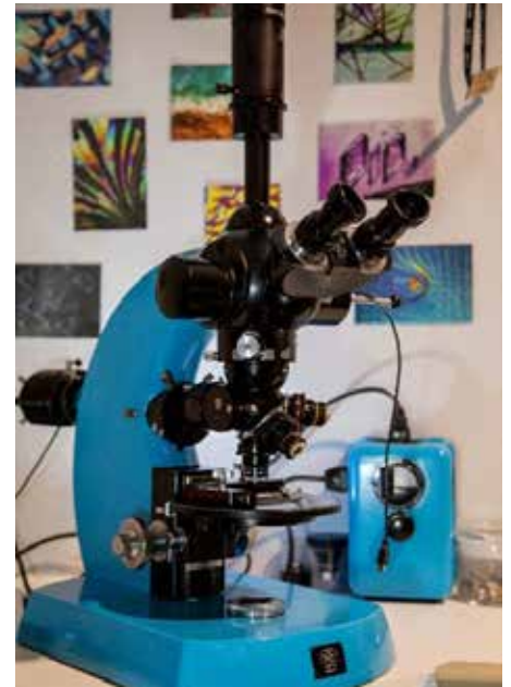
1. Left: The author's Nikon SMZ10 stereomicroscope with gemmological base and fibre-optic illumination setup. Right: The author's custom vintage Zeiss Universal compound microscope equipped with differential interference contrast (DIC) components, which facilitates the examination of surfaces of gem materials at high resolution.
