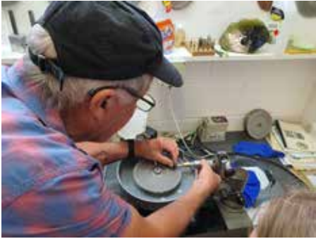
Richard Ussher (left) shows how to shape the material – in this case, green glass – using a lap, once the specimen is mounted on a dop (right).
