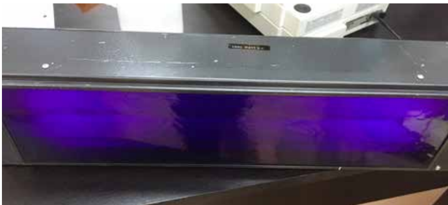
Phosphor-coated glass tube (historically used in long-wave UV radiation).
