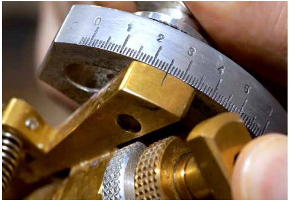
3: The faceting handpiece, used to select angles for cutting, is shown set to 25 degrees.
