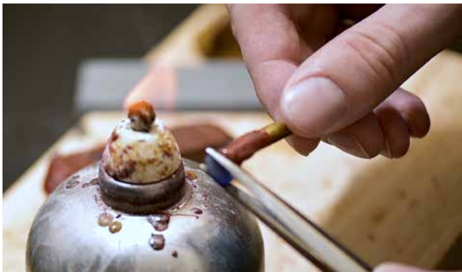
1: Dop wax is used to attach the rough blue spinel crystal to the dop stick.
