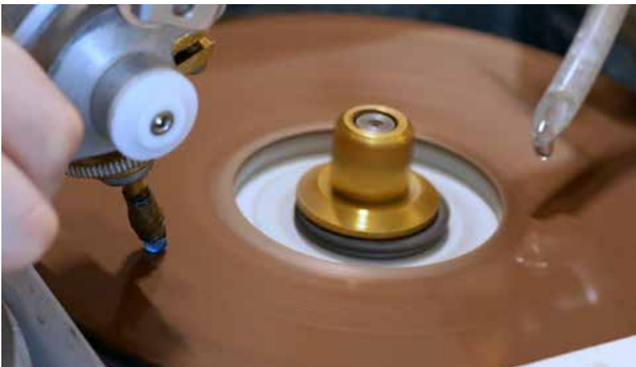
2: Once attached to the dop stick, the spinel is ready for cutting on the first lap.
