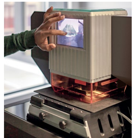
The state-of-the-art LA-ICMPS facility at the Gübelin Gem Lab collects a huge amount of chemical data on each stone.
