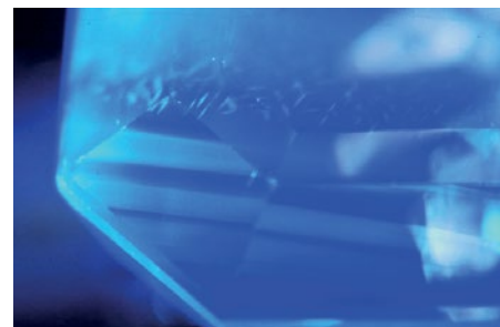
These photomicrographs show dust bands in three different blue sapphires from Kashmir (left), Sri Lanka (centre) and Madagascar (right), exemplifying the similarity of microscopic features that can be found in sapphires from different origins. Such similarities of microscopic properties forced gem labs to reach out to more sophisticated analytics, to keep up the origin determination service.
