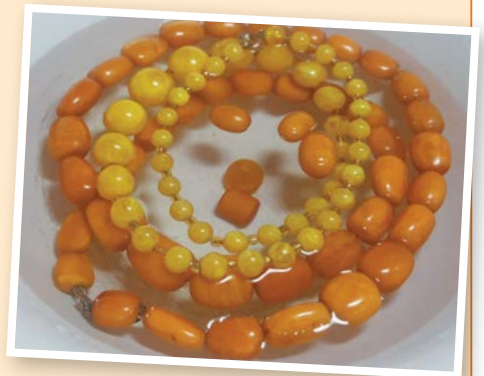
4: Testing both the amber and plastic in salt water, with the plastic and amber strung beads floating, three loose amber beads floating and two plastic imitations sunk at the bottom (as distinguished by the shadows of those above cast downwards).
