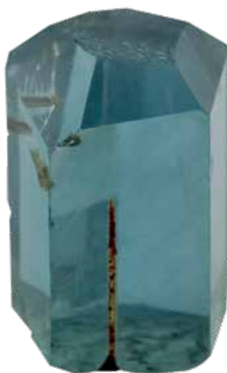
11a: This blue specimen presented as aquamarine was a synthetic quartz fashioned into a hexagonal crystal, terminated by pyramidal and pinacoidal faces. Also note the conical tube containing brown epigenetic substance.
