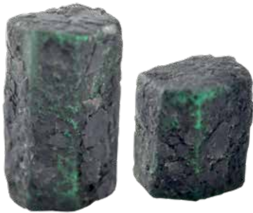
4: These glass samples are worked-up to imitate emerald rough, by fashioning into hexagonal crystals and coating with black mica; these were found mixed in a parcel of natural emerald.
