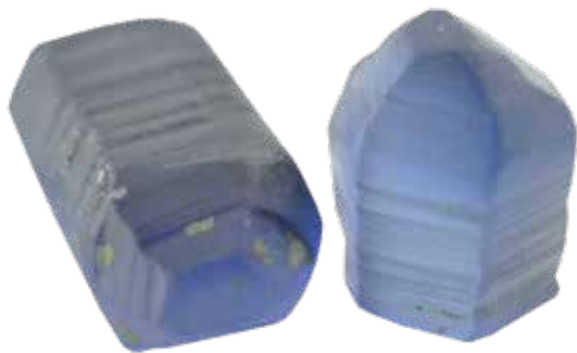
7: Presented as natural sapphire, these specimens (a & b) were turned out to be synthetic. These were presented as broken, tumbled rough (7a top, and as fashioned, well-formed hexagonal-pyramidal crystals with surface markings (7b above).
