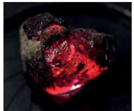
6: This bright purplish red-pink rough (6a left) is a composite made up of synthetic and natural ruby. The central part is a synthetic ruby while the outer part is composed of chips of natural ruby. Note the small areas of angular milky zones. Under transmitted light (6b right, central synthetic part of the specimen appeared bright red, while the edges appeared dark and opaque.
