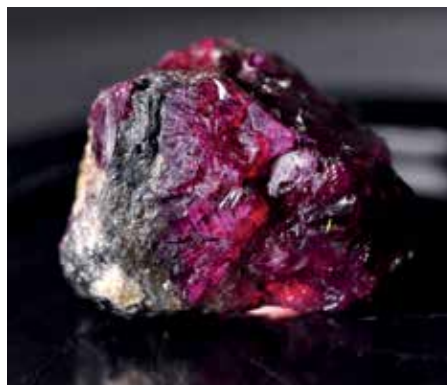
6: This bright purplish red-pink rough (6a left) is a composite made up of synthetic and natural ruby. The central part is a synthetic ruby while the outer part is composed of chips of natural ruby. Note the small areas of angular milky zones. Under transmitted light (6b right, central synthetic part of the specimen appeared bright red, while the edges appeared dark and opaque.
