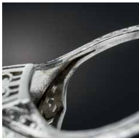
1. Examples of seams and visible joins on die-struck platinum jewellery.
