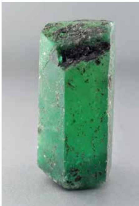
10b: This quartzite specimen, presented as emerald rough was first dyed, then fashioned as hexagonal crystal and randomly coated with black mica.
