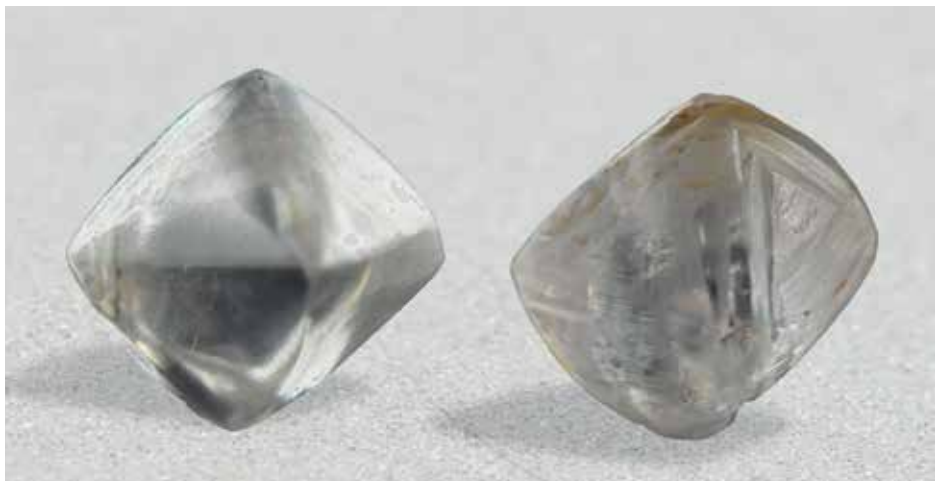
9: These colourless octahedrons, representing diamond, are fashioned cubic zirconia (left) and topaz (right). Also note artificially drawn triangular growth markings on octahedral faces, along with iron-stained films in topaz crystal.
