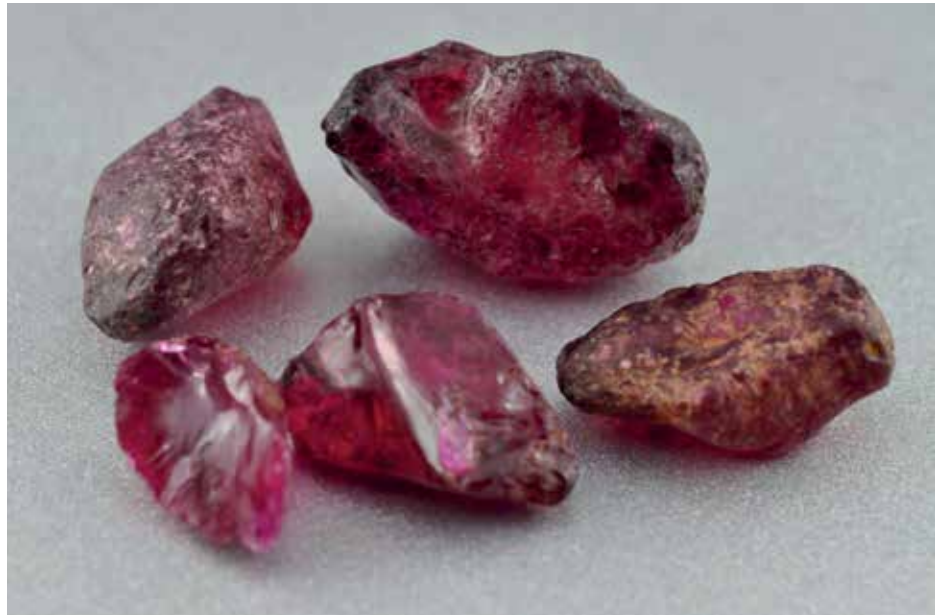
5: These rough specimens weighing 3.60 - 18.06 ct were identified as synthetic ruby. Similar synthetic samples in larger sizes were also encountered earlier, which were said to be purchased from mining areas in Mozambique. Also note the presence of yellow-brown substance on extreme right specimen, imitating mud on natural rough.
