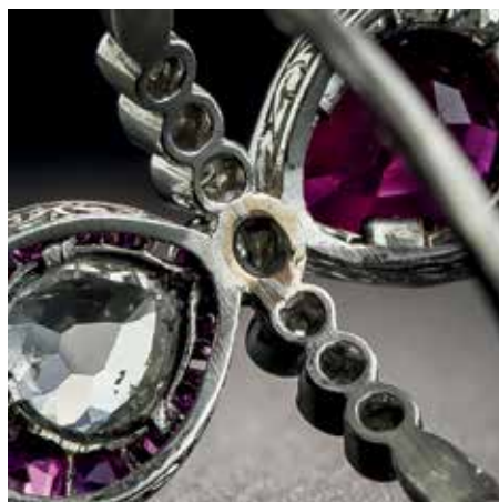
1. Examples of seams and visible joins on die-struck platinum jewellery.
