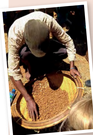
8. Sifting through the illam yield at Elahera mine.
