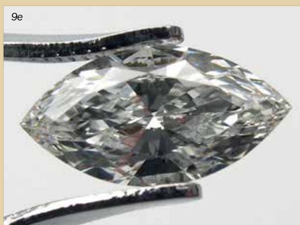
9 (e-g) Marquise-cut diamond, 0.52 ct, displaying reflections from the laser number on the girdle, magnification approx. 7×, 25× and 60×.
