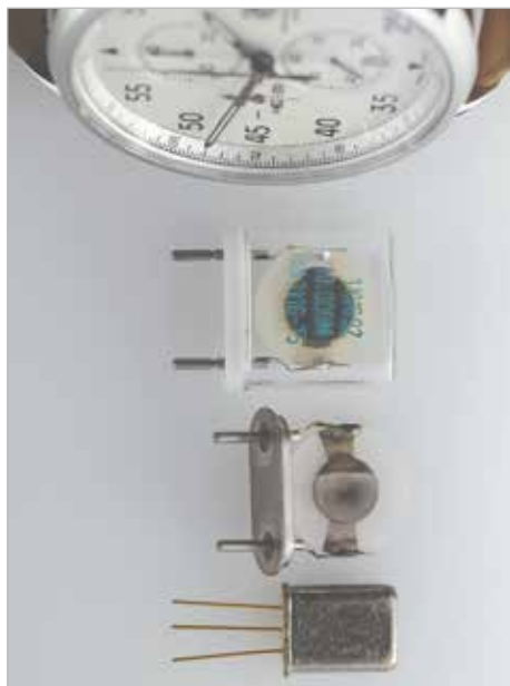
A quartz watch and three different oscillating quartz crystals with electrodes in different frequencies.
