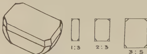
FIG. 76. Shape Correct proportions the preform like a —always in milli- "Dutch barn." meters.
