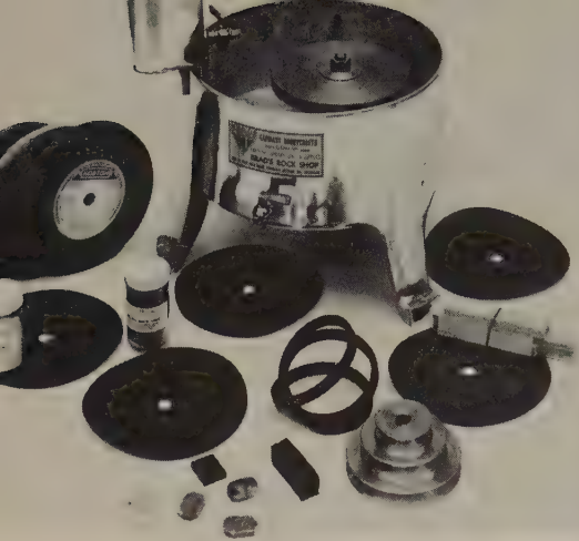
FIG. 25. Gemlap horizontal unit. Comes complete with grinding wheels, iron lap, sanding disks, felt polishing disk, grit, polishing powder, pulley and belt. (No motor.)
