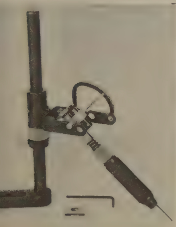
FIG. 62. The Lee faceting unit features a lift-off handpiece, positive guide device by which a gem may be turned accurately, sturdy construction and low cost.
