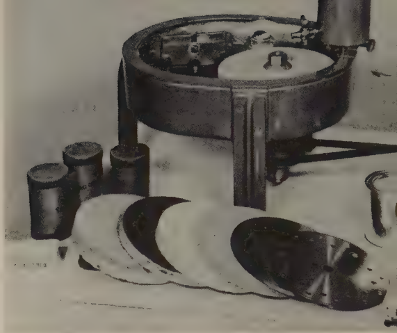
FIG. 26. B & I Gem Maker. Comes complete with grinding wheel, swing vise, diamond saw blade, iron lap, felt disk, diamond sticks and cement, grits, polishing powder and gem material. (No motor.)
