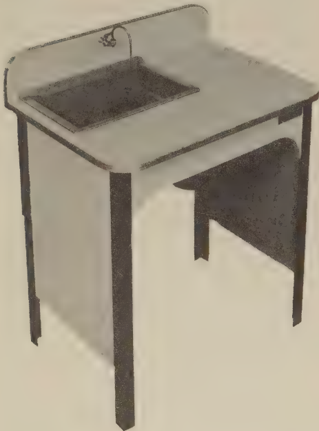
FIG. 58. A faceting table of the type used with the Lee Facet Head.
