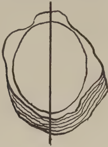
FIG. 46. Mark a long axis on the front, back, and edges of the blank. Next mark the rough outline on the back of the stone, aligning as shown here.
