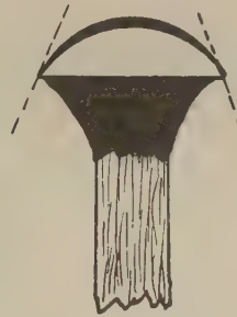
FIG. 37. 3rd step: Completing the arc.
