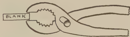
FIG. 22. A pair of ordinary extension pliers can be used for "nibbling" edges of blanks.
