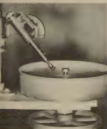
FIG. 65. The Allen faceting unit includes a sturdy, well-made, inexpensive head with all essential features, and can be had with master lap, spindle, and pulley.
