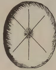
FIG. 44. Orienting star beryl (aquamarine). Note that one ray is placed parallel to the longest dimension of the stone.
