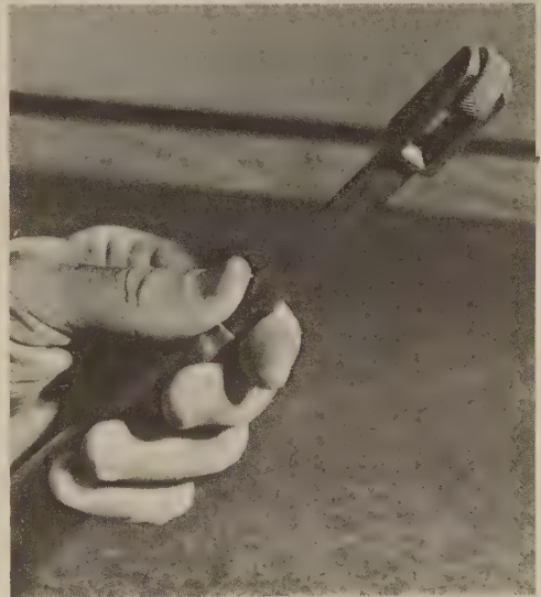
FIG. 72. A scoring wheel for keeping the surface of faceting laps in condition, consisting of a small knurled wheel in a handle.
