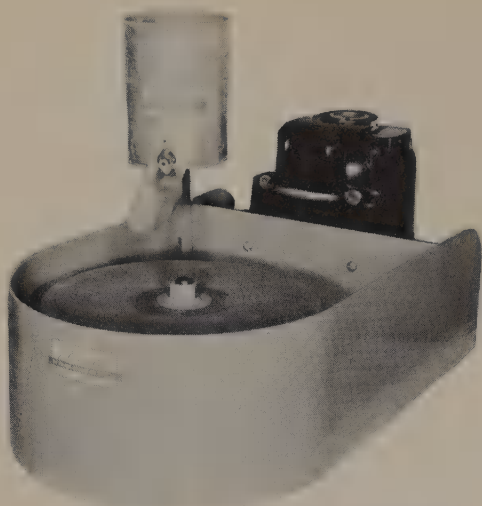
FIG. 98. Covington 10" horizontal lap unit. Available also in 6" or 8" sizes. Comes complete with motor. Completely portable, it has carrying handle. The units use standard grinding wheels, sanders, and buffs. Accessories available include vise, saw, grinding wheel, sanding disk, and polishing buff.
