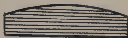
FIG. 45. Cut star beryl to a slight dome. This is a preliminary step in locating a single long ray parallel to the longest diameter of the stone. Oil the surface of the rough-ground and sanded stone and observe under a single ray of light.
