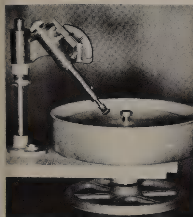
FIG. 65. The Allen faceting unit includes a sturdy, well-made, inexpensive head with all essential features, and can be had with master lap, spindle, and pulley.
