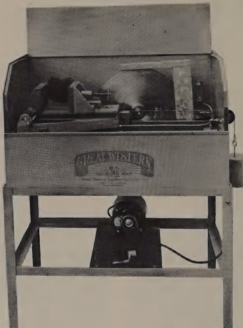
FIG. 4. A Great Western hydraulic-feed slabbing saw, 20" model.
