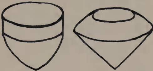
FIG. 74. Preform . . . not cone-shaped should look like this . . . like this.
