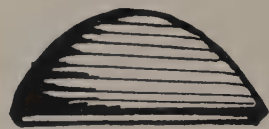
FIG. 48. Cross section—end of stone. Note that the shape is an arc rather than a curve.
