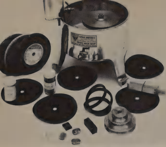
FIG. 25. Gemlap horizontal unit. Comes complete with grinding wheels, iron lap, sanding disks, felt polishing disk, grit, polishing powder, pulley and belt. (No motor.)
