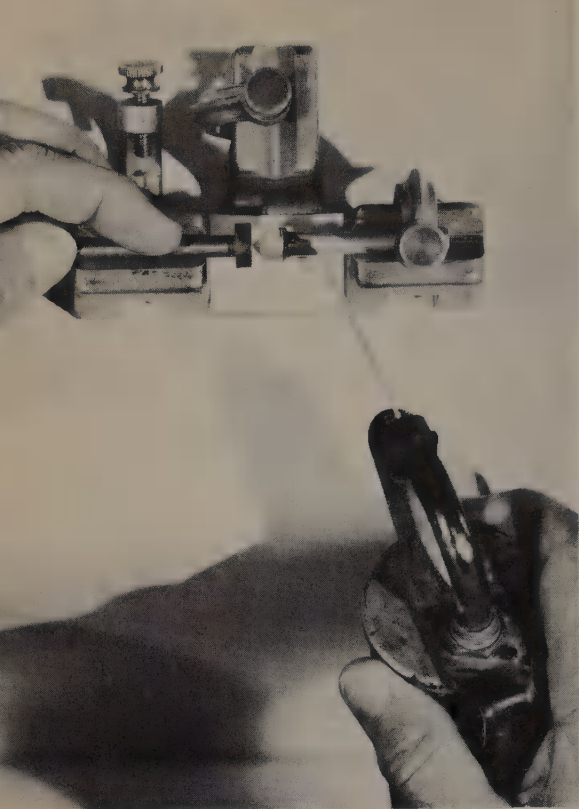
FIG. 77. Step 1: Leveling stone on the dop.
