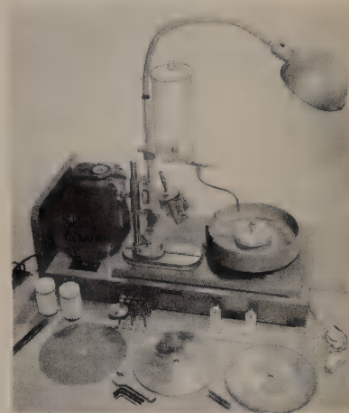
FIG. 64. The Graves faceting unit is a deluxe outfit that is very accurate and is self-contained. The outfit shown has everything needed—just plug it in and facet.
