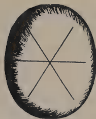
FIG. 43. Orienting the rays of star sapphire. Note that one ray is directly across the shortest dimension of the stone.
