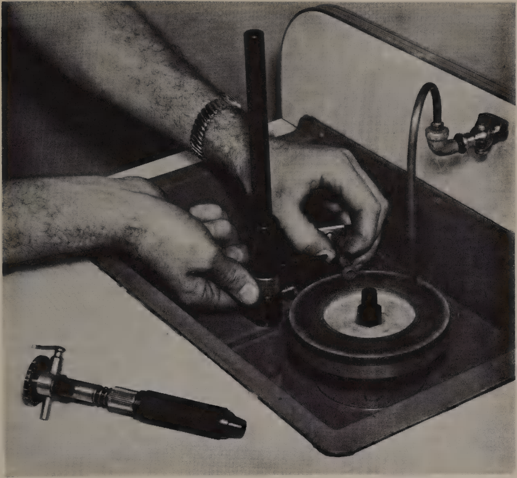
FIG. 83. One of several methods for grinding a brilliant preform round.
