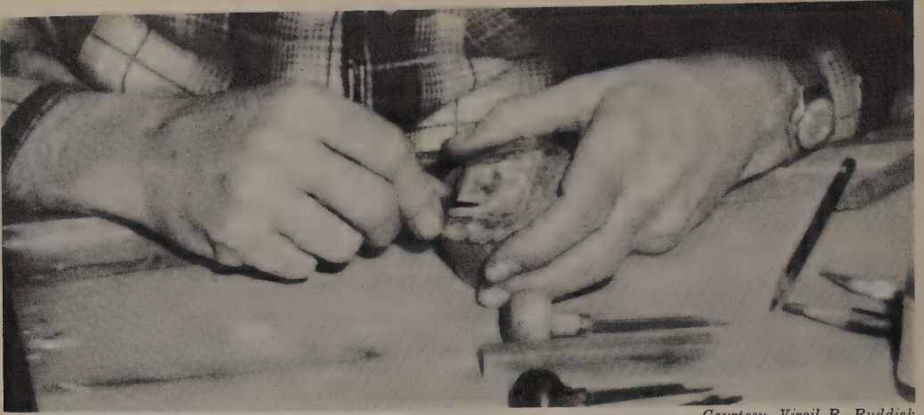
FIG. 133. Cutting lines in fins using two-line graver.
