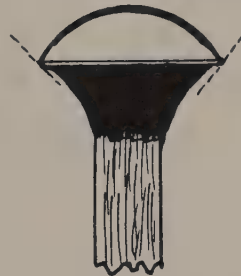
FIG. 38. 4th step: Back beveling.
