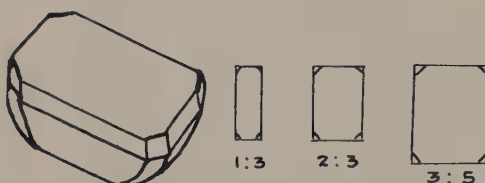
FIG. 76. Shape the preform like a "Dutch barn." Correct proportions —always in millimeters.
