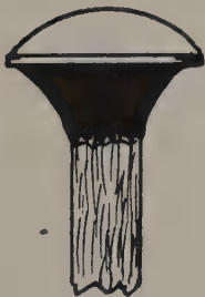
FIG. 36. 2nd step: Rounding the top.
