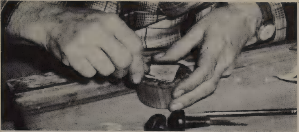
FIG. 130. Cutting outlines with a round graver.
