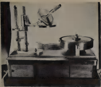
FIG. 59. The O'Brien portable faceting unit makes use of a simplified octagonal plate resting freely on a flat metal table with which to index the positions for cutting gems. The base contains the motor.
