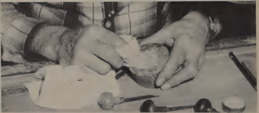
FIG. 135. Polishing with cerium oxide.
