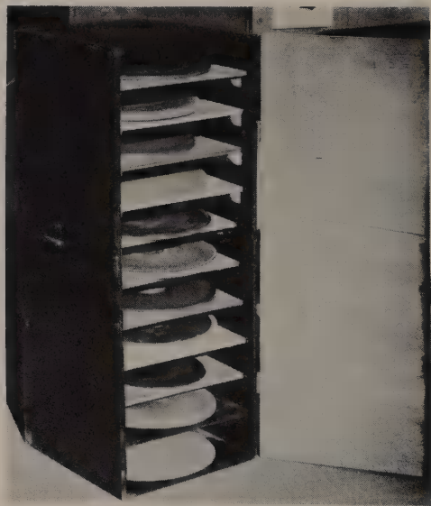
FIG. 69. A lap storage cabinet to prevent contamination of faceting and polishing laps by foreign matter, grit, etc.
