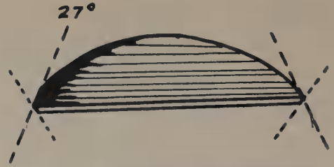
FIG. 47. Cross section—side of stone.
