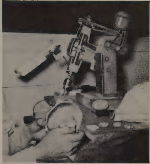
FIG. 102. An adjustable carving machine built by R. M. Musick, of Escondido, California, using standard bearings and parts. The machine can be tilted to any angle.
