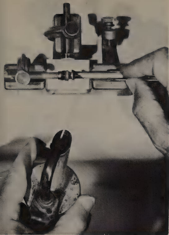
FIG. 81. Step 5: Separating the gem from the first dop. The stone has now been turned.
