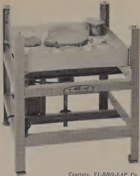
FIG. 100. A vibratory lapping machine.
