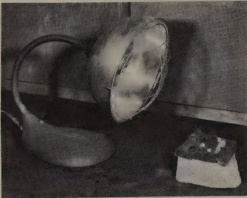
FIG. 82. Use a heat lamp and a pad of steel wool for dopping sensitive gems.
