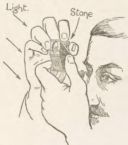
FIG. 17.—Method of Using the Refractometer.
