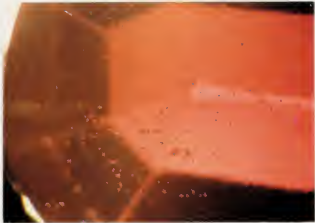
Profilated bubbles in synthetic ruby
