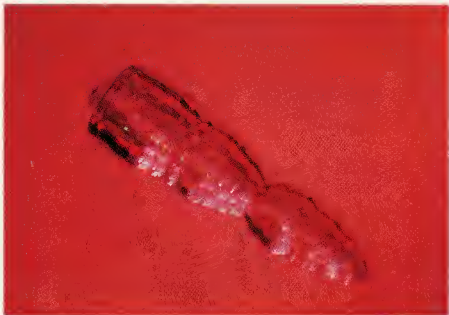
Bubble in flame-fusion synthetic ruby (50X)
