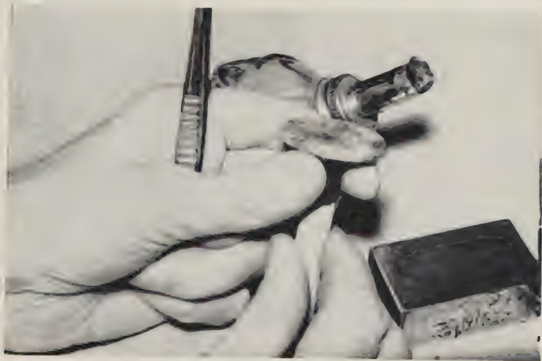
Cut 31. Dopping the Roughed-Out Stone. The fingers work up the dopping cement to form a supporting shelf for the overhang of the stone.
