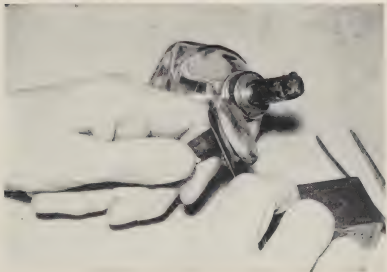
Cut 35. Undopping the Cabochon. Removing the gem from the dop stick is simple enough, but many stones are cracked or broken because the cutter pried the stone from the cement. The way to do it is to pry the cement away from the stone.
