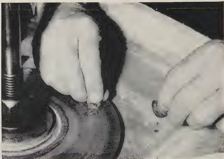
Cut 2. When cutting facets the table is the first facet to be cut, as shown here. The wheel is bell metal bronze impregnated with diamond dust.
