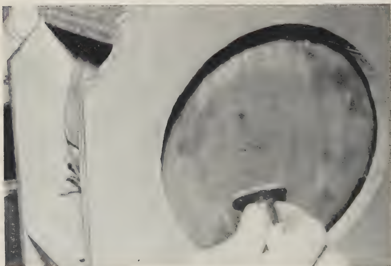
Cut 33. Smoothing the Gem Stone. A padded disc is covered with carborundum cloth of 220 grit, and the stone is gently stroked against it while the disc runs at moderate speed. The gem is kept constantly in motion by twisting as well as stroking to avoid overheating.
