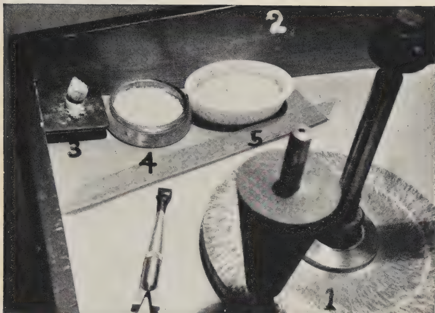
Figure 80. Polishing-Agent and Wetting-Plug Assembly. 1, polishing lap; 2, guard rail; 3, block with wetting plug; 4, polishing agent; 5, water. (Notice that this lap is scored with pits instead of lines).
