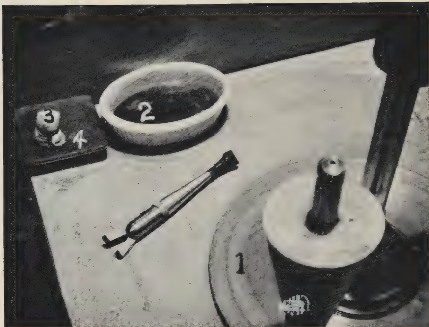
Figure 70. Assembly for Watering the Diamond Lap (view from above). 1, cutting lap; 2, water receptacle; 3, cloth wetting plug; 4, base for plug when not in actual use.
