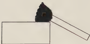
Figure 29. Cabochon Dop Stick With a Mass of Cement on a Rolling Block, Being Rolled Into the Proper Cone for Receiving Roughed-Out Stone.
