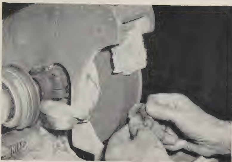
Cut 30. Rough Grinding the Cabochon. The purpose is to give the gem stone the general shape, size, and contour desired. Note the manner of holding the stone against the wheel.
