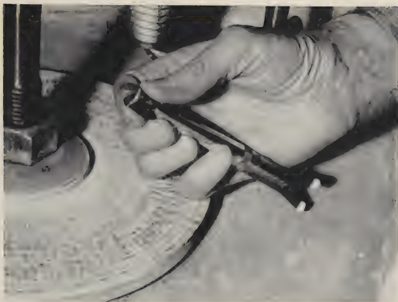
Cut 8. Inspecting the progress of polishing. Shown here is the correct manner of holding the device—the tips of the thumb and forefinger next to the stone, the other three on the device.
