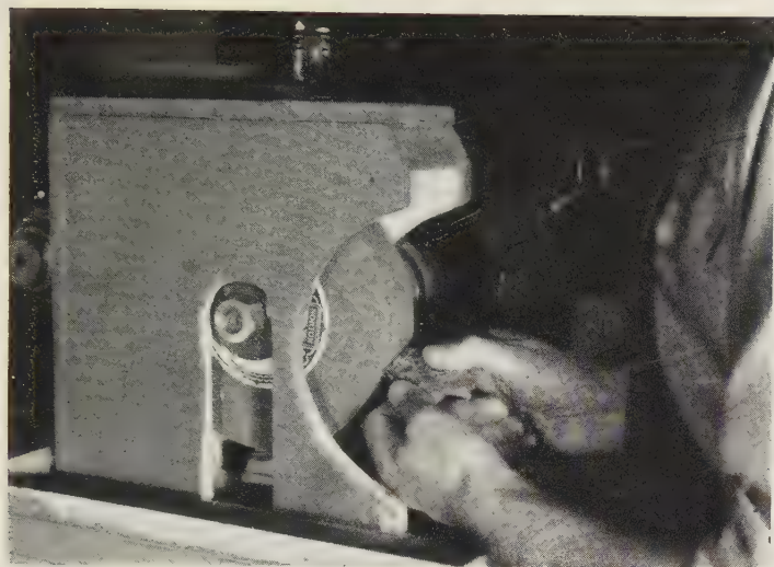
Figure 19. Grinding the Rough Stone. The direction of the grinding wheel is clockwise when viewed from the left side of the wheel. Note the manner of holding the stone to the wheel.
