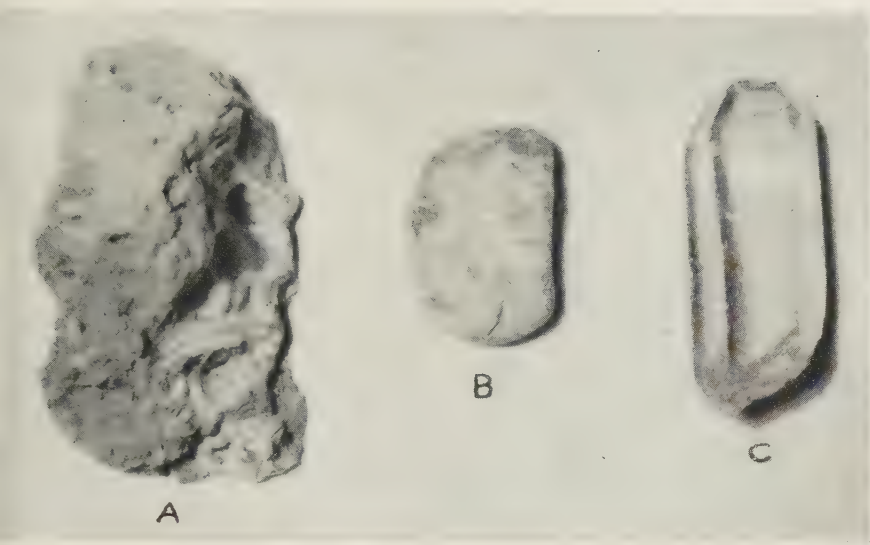
Figure 4. Forms of Rough Gem Material. A, irregular chunk or block; B, water-worn pebble; C, quartz crystal.
