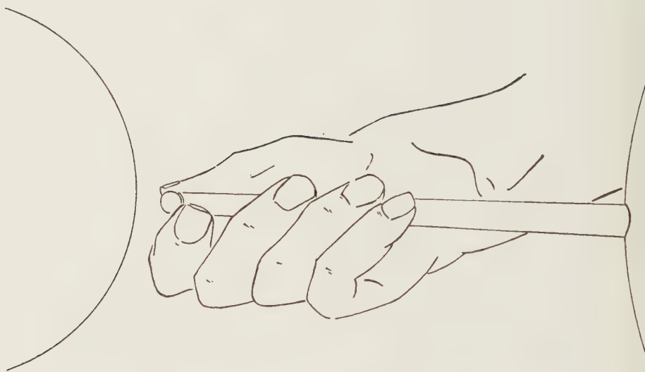
Figure 84. Cutting a Bead With Breastplate and Stick. Cutting wheel, bead, stick with cupped end, and breastplate.
